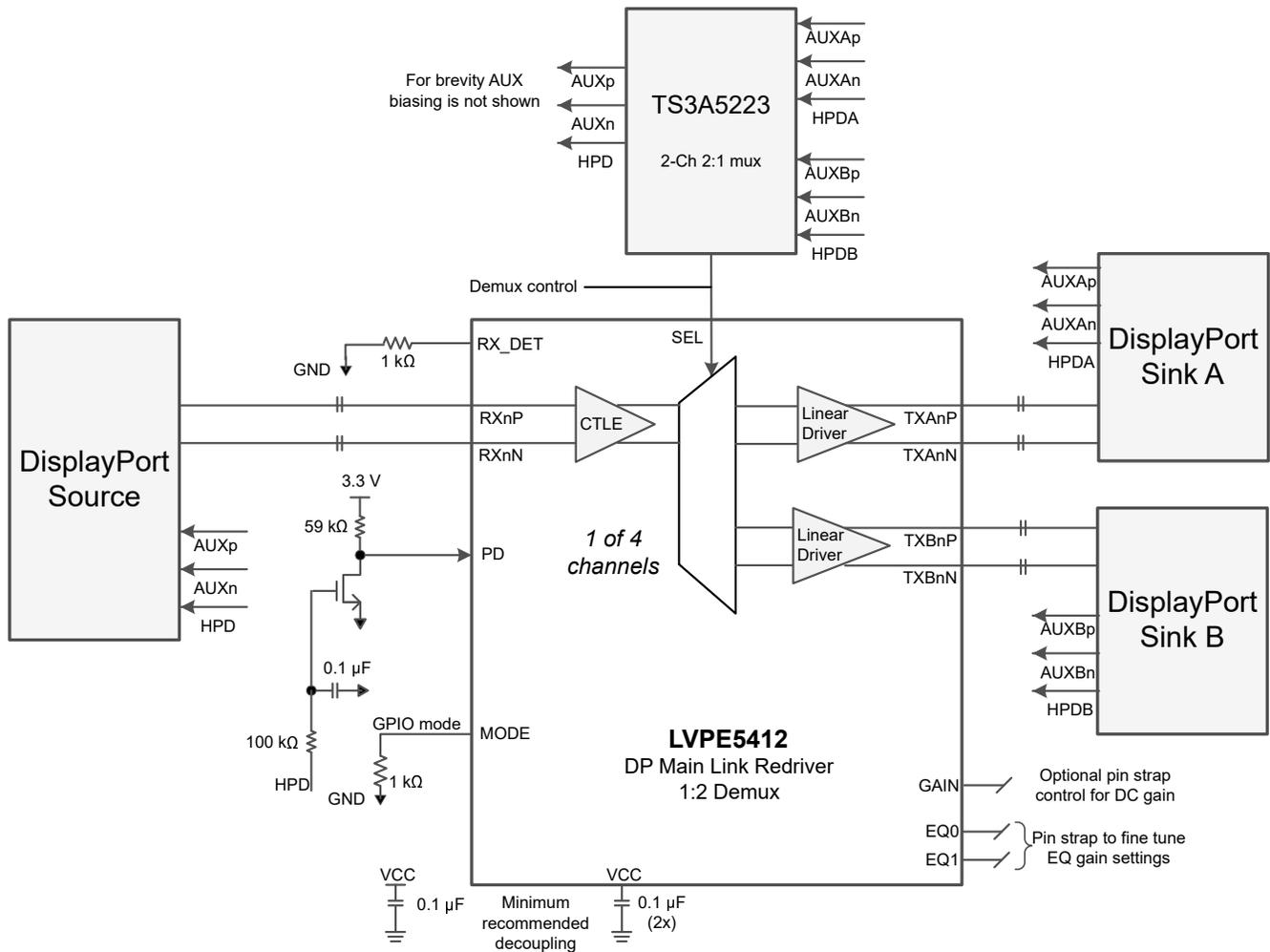
图 7-2. Simplified Schematic for DisplayPort Demultiplexer Application
