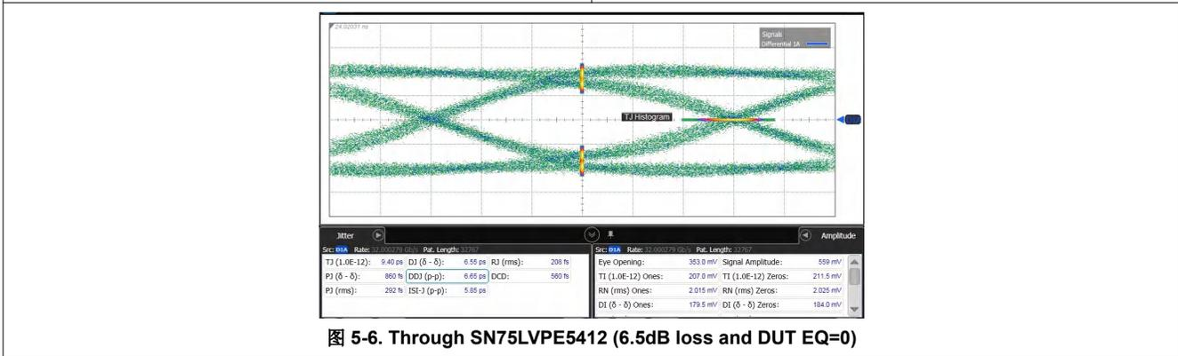
图 5-6. Through SN75LVPE5412 (6.5dB loss and DUT EQ=0)
