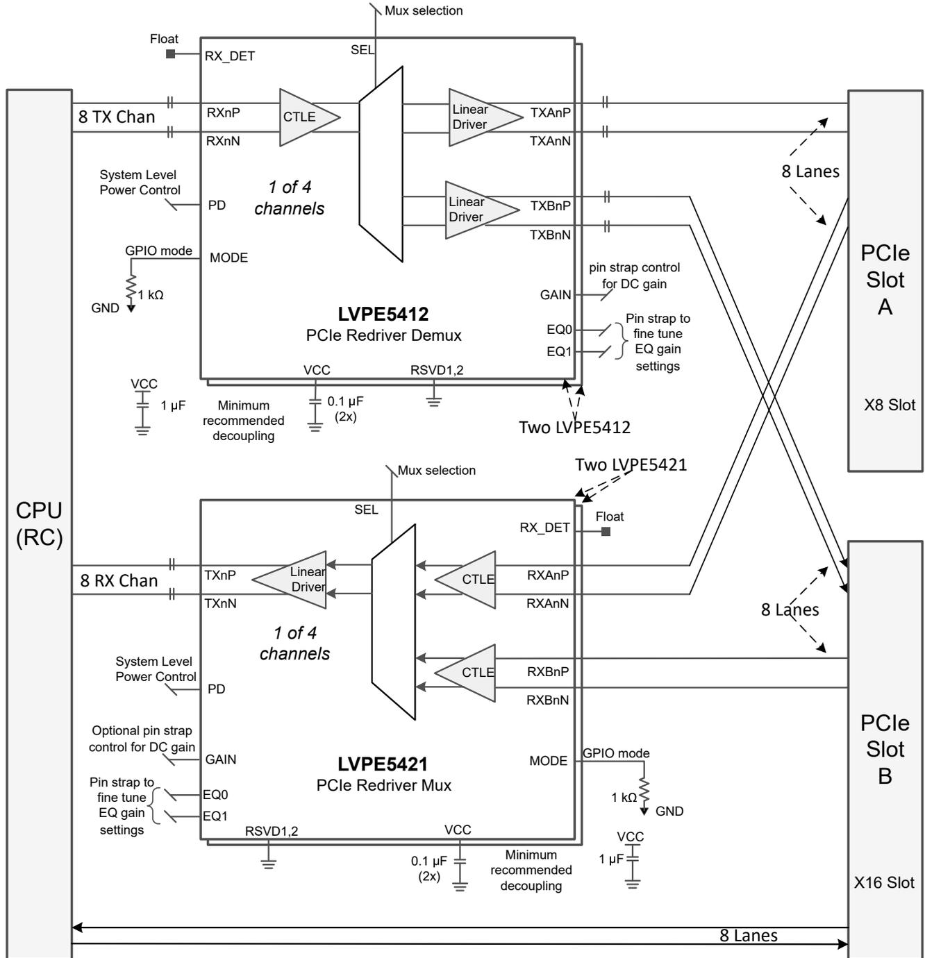
图 7-1. Simplified Schematic for PCIe Lane Switching
