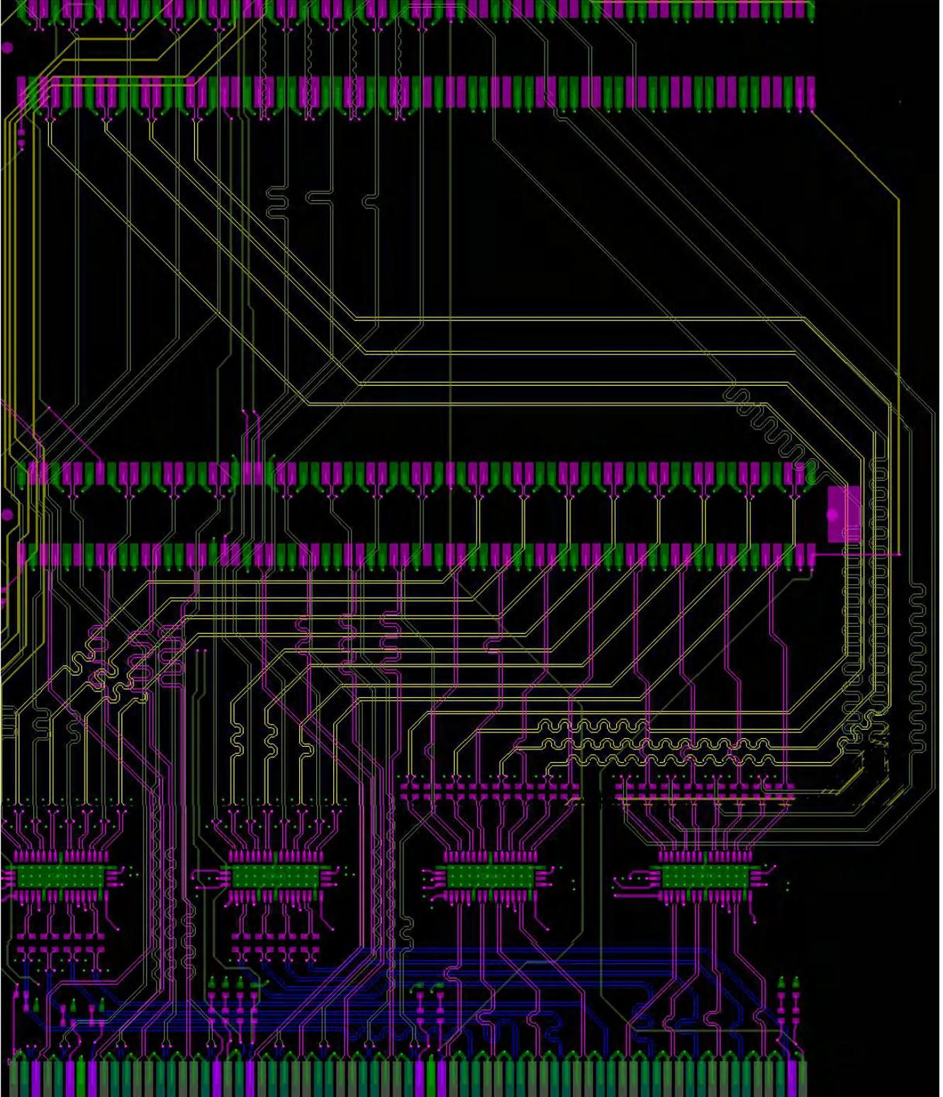
图 7-4. Layout Example for PCIe Lane Muxing Application
