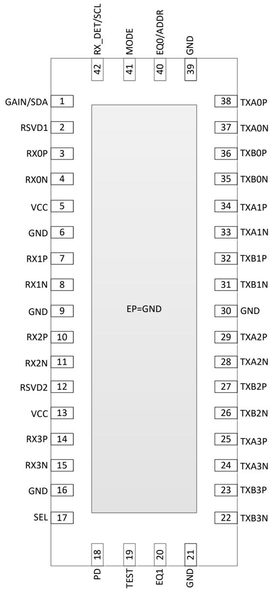
图 4-1. RUA Package, 42-Pin WQFN (Top View)
