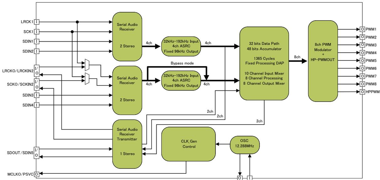
图 47. Digital Audio Signal Flow Block Diagram
