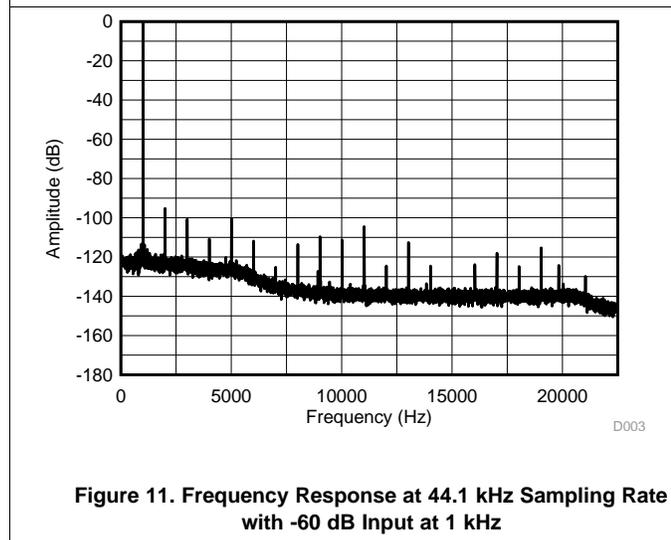
Figure 11. Frequency Response at 44.1 kHz Sampling Rate with -60 dB Input at 1 kHz
