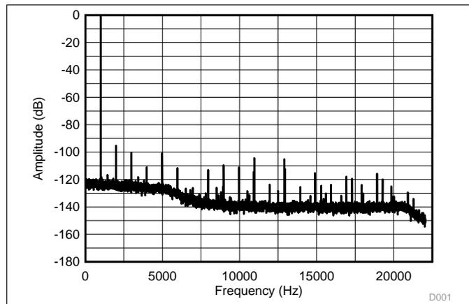
Figure 9. Frequency Response at 48 kHz Sampling Rate with -60 dB Input at 1 kHz
