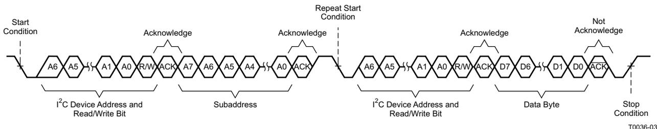
Figure 43. Single-Byte Read Transfer
