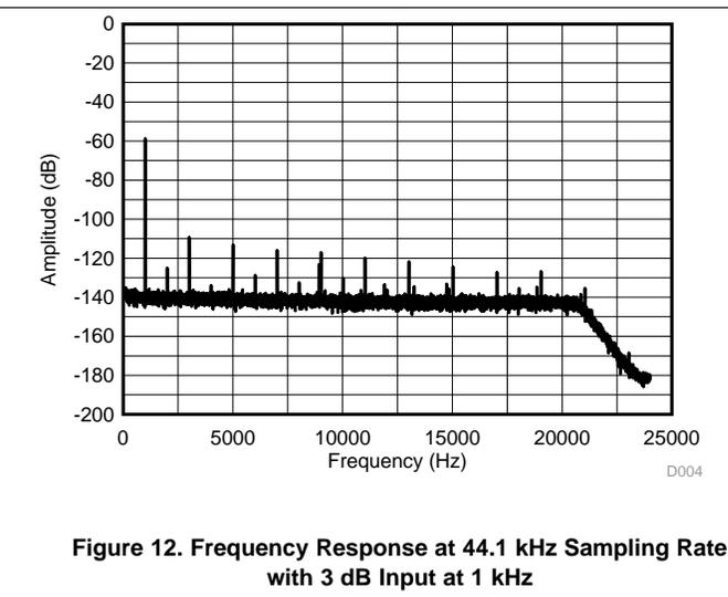
Figure 12. Frequency Response at 44.1 kHz Sampling Rate with 3 dB Input at 1 kHz
