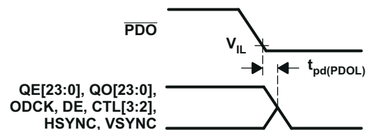
图 6-7. Delay From \overline{\text{PDO}} Low to Hi-Z Outputs
