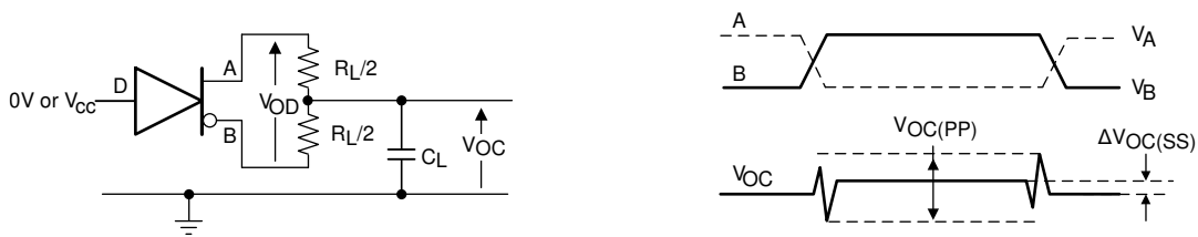
图 7-2. Measurement of Driver Differential and Common-Mode Output With RS-485 Load
