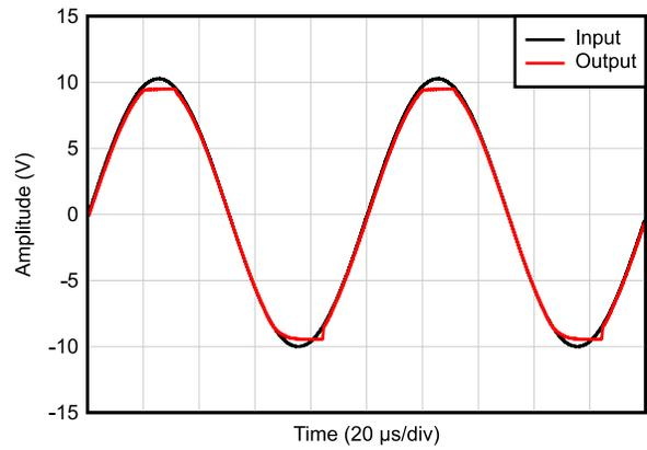
$V_S = \pm 10\text{V}$ ,  $V_{IN} = V_{OUT}$
