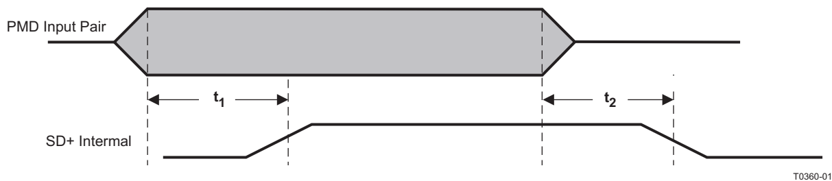
Figure 9-20. 100Base-TX Signal Detect Timing
