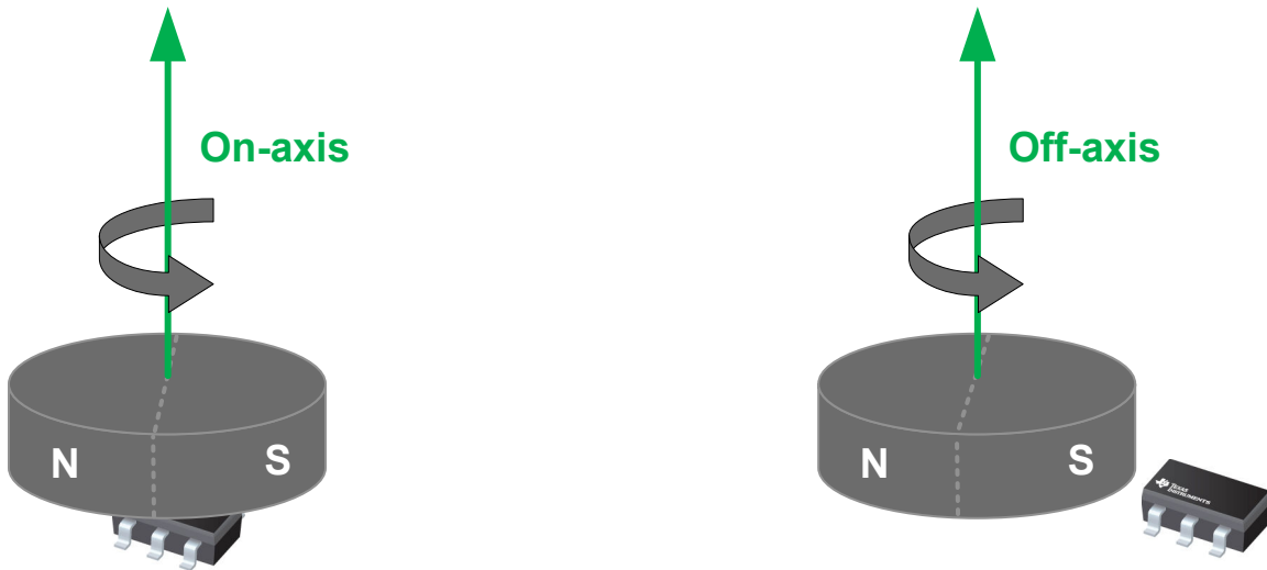
图 8-11. On-Axis vs Off-Axis Angle Measurements
