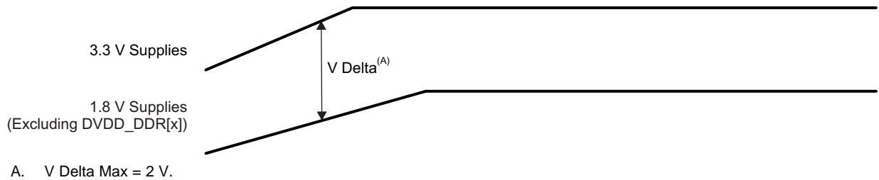
Figure 7-2. 3.3 V Supplies Rising Before 1.8 V Supplies Delta
