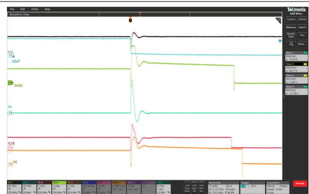
器件处于稳定状态，OUT 短接至 GND。Vin = 51V。C<sub>out</sub> = 3uF
