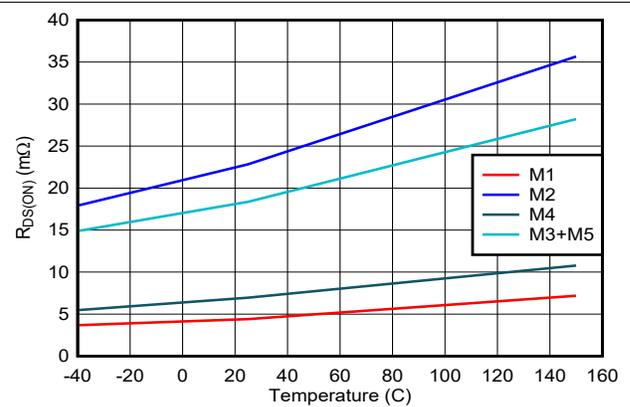
图 7-16. Buck-Boost Power FET  $R_{DS(ON)}$  vs Temperature
