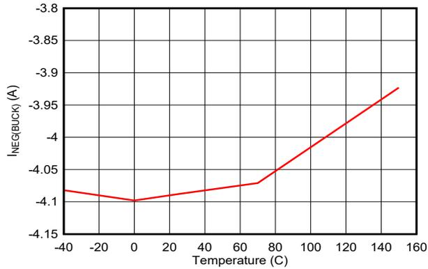
图 7-21. Buck Negative Current Limit vs Temperature
