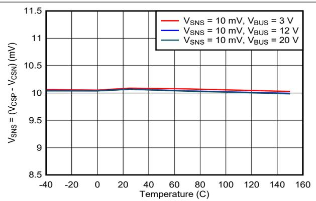
Target  $V_{SNS}$  for Current Limit = 10 mV
