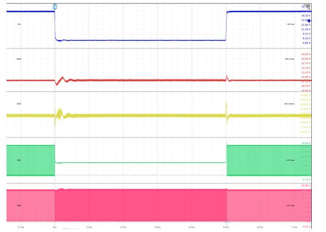
$V_{IN} 7V \rightarrow 18V$        $V_{BUS} = 20V$        $I_{BUS} = 3A$
