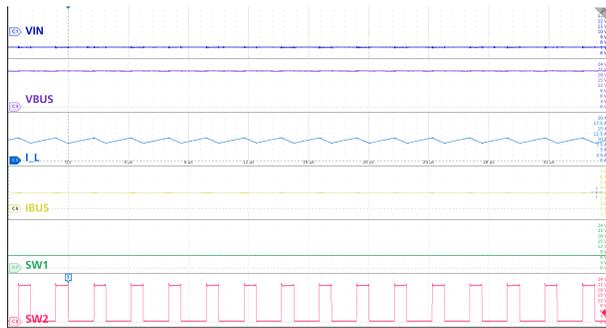
$V_{IN} = 7\text{ V}$       $V_{BUS} = 20\text{ V}$       $I_{BUS} = 3\text{ A}$
