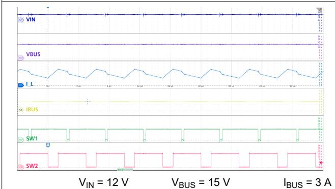
图 10-26. Buck-Boost Mode: Nominal  $V_{IN}$ , 3 A Load
