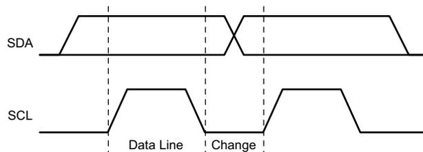
图 9-36. I<sup>2</sup>C Bit Transfer
