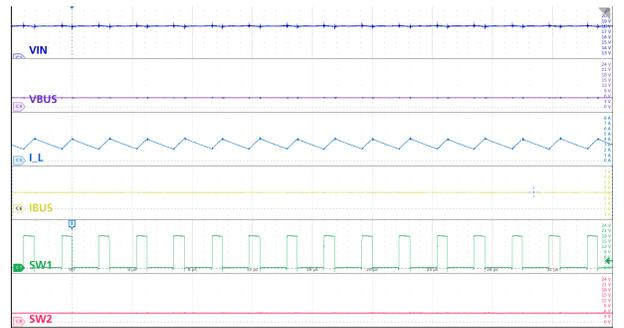
$V_{IN} = 18\text{ V}$       $V_{BUS} = 5\text{ V}$       $I_{BUS} = 3\text{ A}$
