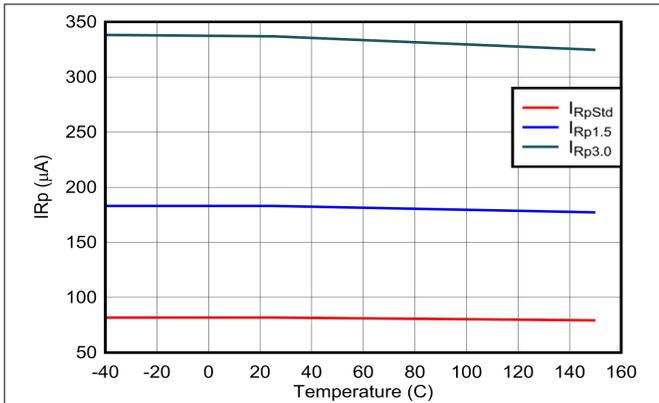
图 7-37. Type-C Cable Detect:  $I_{Rp}$  vs Temperature
