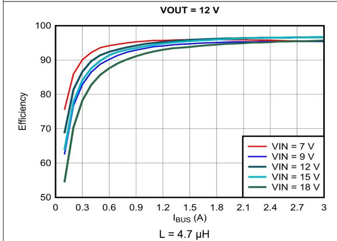
图 10-8. Efficiency vs Output Current ( $I_{OUT}$ ),  $V_{OUT} = 12\text{ V}$
