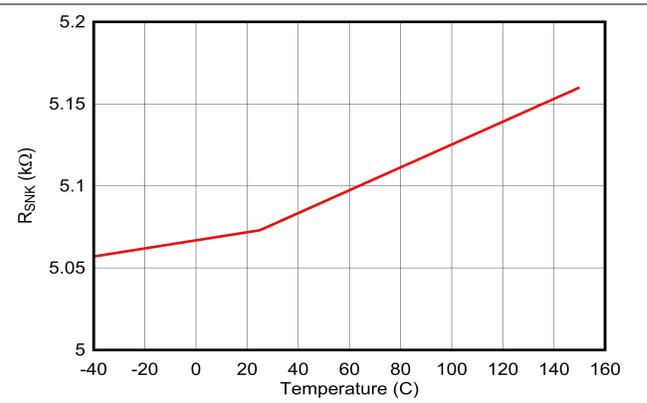
图 7-38. Type-C Cable Detect:  $R_{SNK}$  vs Temperature
