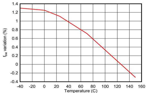
图 7-24. Buck-Boost Switching Frequency Variation vs Temperature
