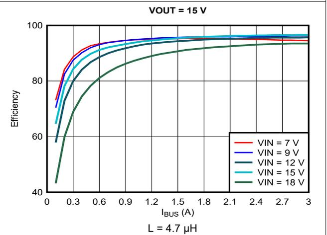
图 10-9. Efficiency vs Output Current ( $I_{OUT}$ ),  $V_{OUT} = 15\text{ V}$
