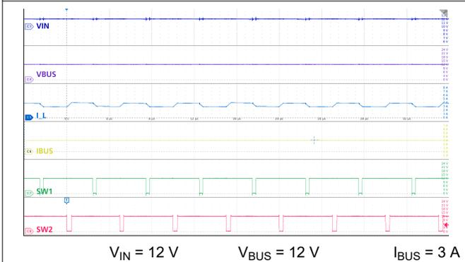
图 10-24. Buck-Boost Mode:  $V_{IN} = V_{BUS}$ , 3 A Load
