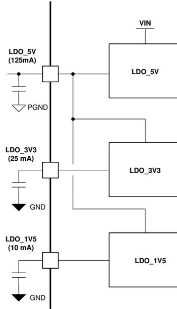
Note: LDO\_5V max regulation current includes LDO\_3V3 (25 mA) and LDO\_1V5 (10 mA)
