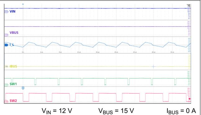
图 10-25. Buck-Boost Mode: Nominal  $V_{IN}$ , No Load
