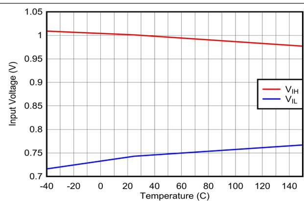
图 7-48. GPIO: Input Voltage Thresholds vs Temperature
