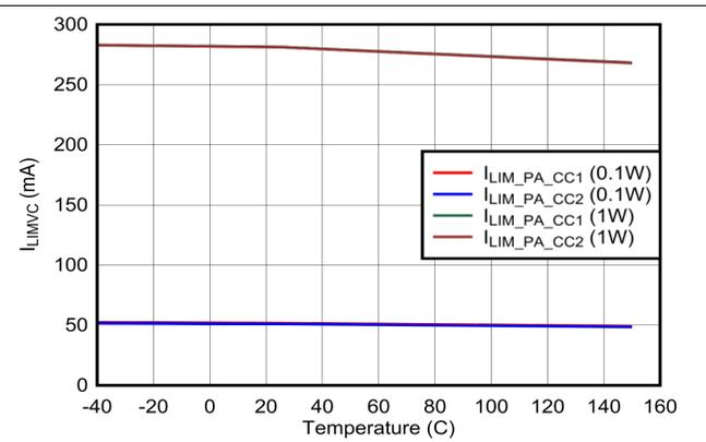
图 7-40.  $V_{CONN}$  Power Path: Current Limit vs Temperature
