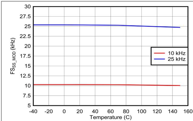
Figure 7-25.  $f_{sw}$  Dither Modulation Frequency vs Temperature
