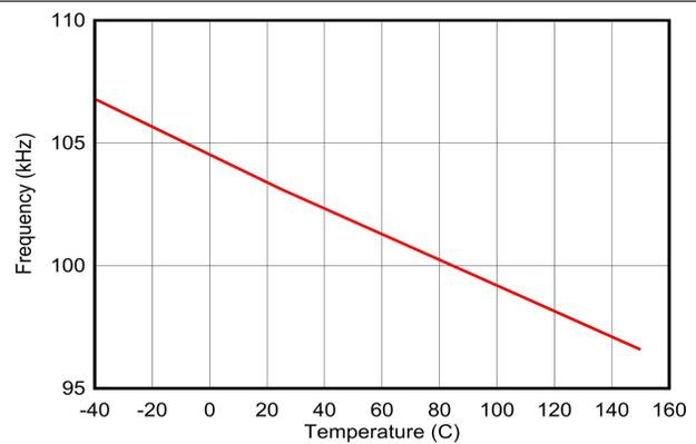
图 7-36. (M0) 100 kHz Oscillator vs Temperature
