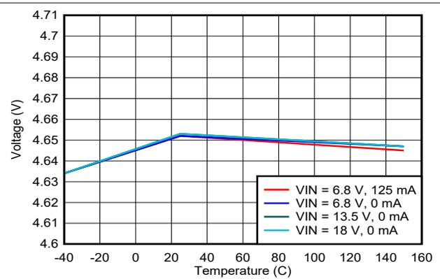
图 7-8. LDO\_5V vs  $V_{IN}$  and Temperature
