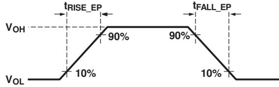
**图 8-3. USB Endpoint Transmitter Rise and Fall Time**
