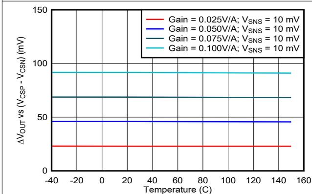
Figure 7-29. Cable Voltage Droop Compensation vs Temperature
