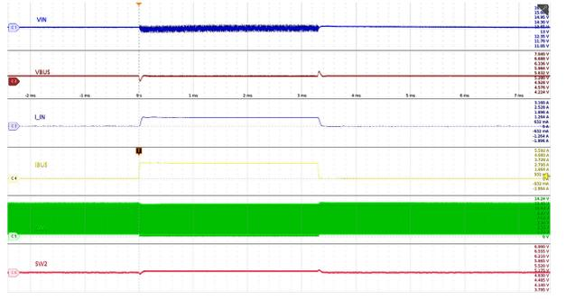
$V_{IN} = 13.5V$        $V_{BUS} = 5V$        $I_{BUS} 0A \rightarrow 3A$
