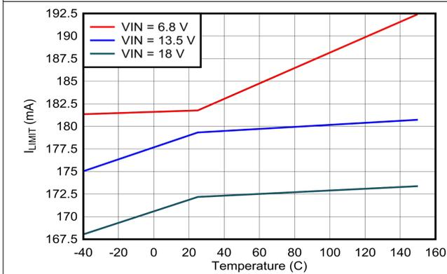
图 7-9. LDO\_5V Current Limit vs  $V_{IN}$  and Temperature
