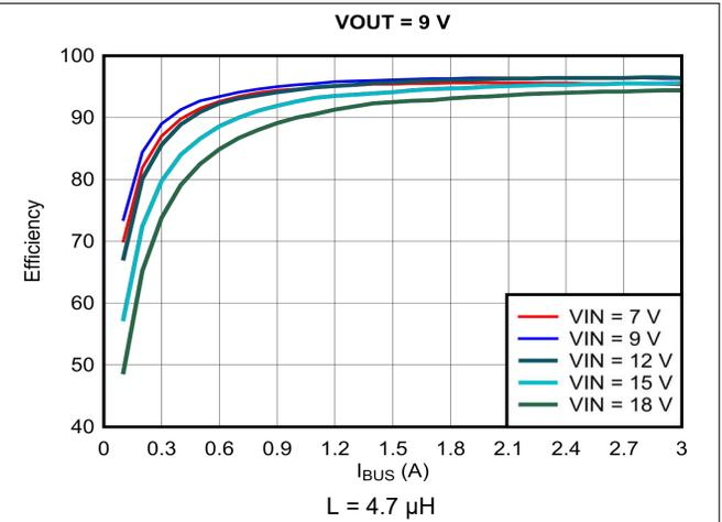
图 10-7. Efficiency vs Output Current ( $I_{OUT}$ ),  $V_{OUT} = 9\text{ V}$
