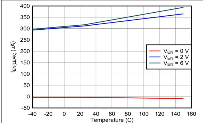
图 7-5. EN Leakage Current vs Temperature
