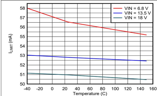
图 7-11. LDO\_3V3 Current Limit vs  $V_{IN}$  and Temperature
