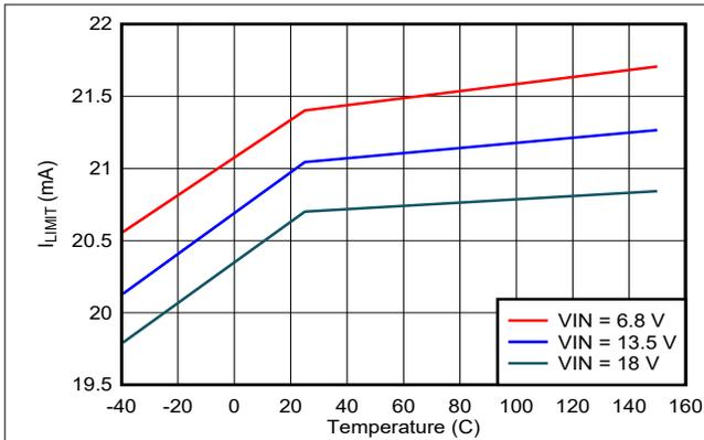
图 7-13. LDO\_1V5 Current Limit vs  $V_{IN}$  and Temperature
