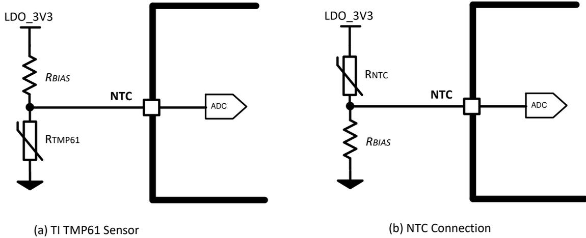
图 9-42. Thermistor Connections (a) PTC, (b) NTC
