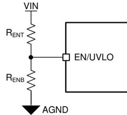
图 9-2. UVLO Threshold Programming
