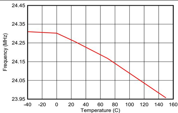
图 7-35. (M0) 24 MHz Oscillator vs Temperature
