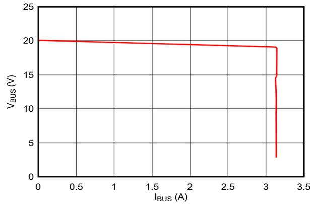
$V_{IN} = 13.5\text{ V}$      $V_{BUS} = 20\text{ V (CV)}$      $I_{LIMIT} = 3.15\text{ A (CC)}$
