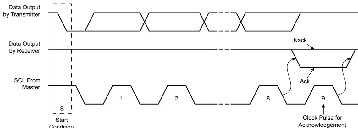
图 9-37. I<sup>2</sup>C Acknowledgment
