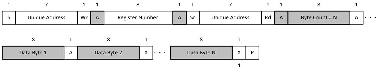
图 9-39. I<sup>2</sup>C Unique Address Read Register Protocol
