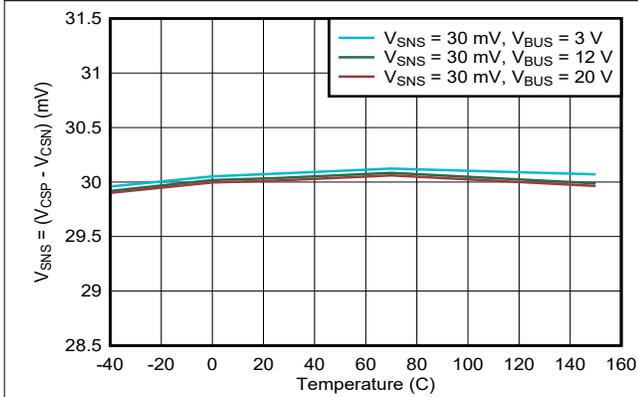
Target  $V_{SNS}$  for Current Limit = 30 mV
