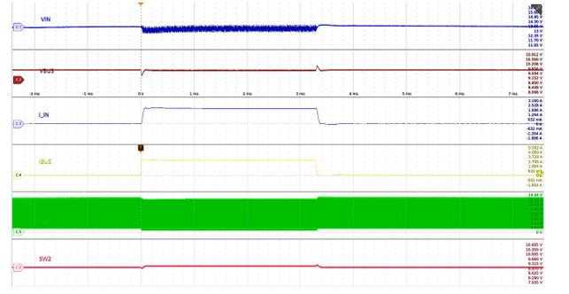
$V_{IN} = 13.5V$        $V_{BUS} = 9V$        $I_{BUS} 0A \rightarrow 3A$
