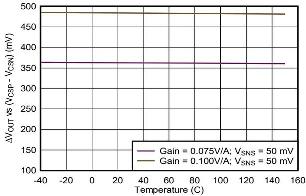
图 7-31. Cable Voltage Droop Compensation vs Temperature
