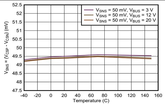
Target  $V_{SNS}$  for Current Limit = 50 mV
