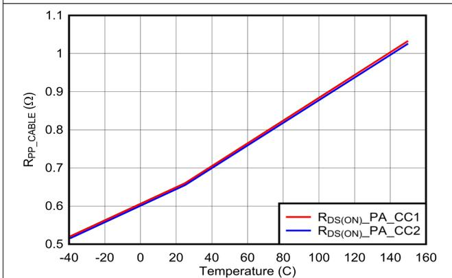
图 7-39.  $V_{CONN}$  Power Path:  $R_{DS(ON)}$  vs Temperature
