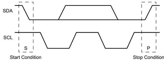
图 9-35. I<sup>2</sup>C Definition of Start and Stop Conditions
