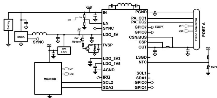
图 10-2. Simplified Single USB PD with MCU/HUB
