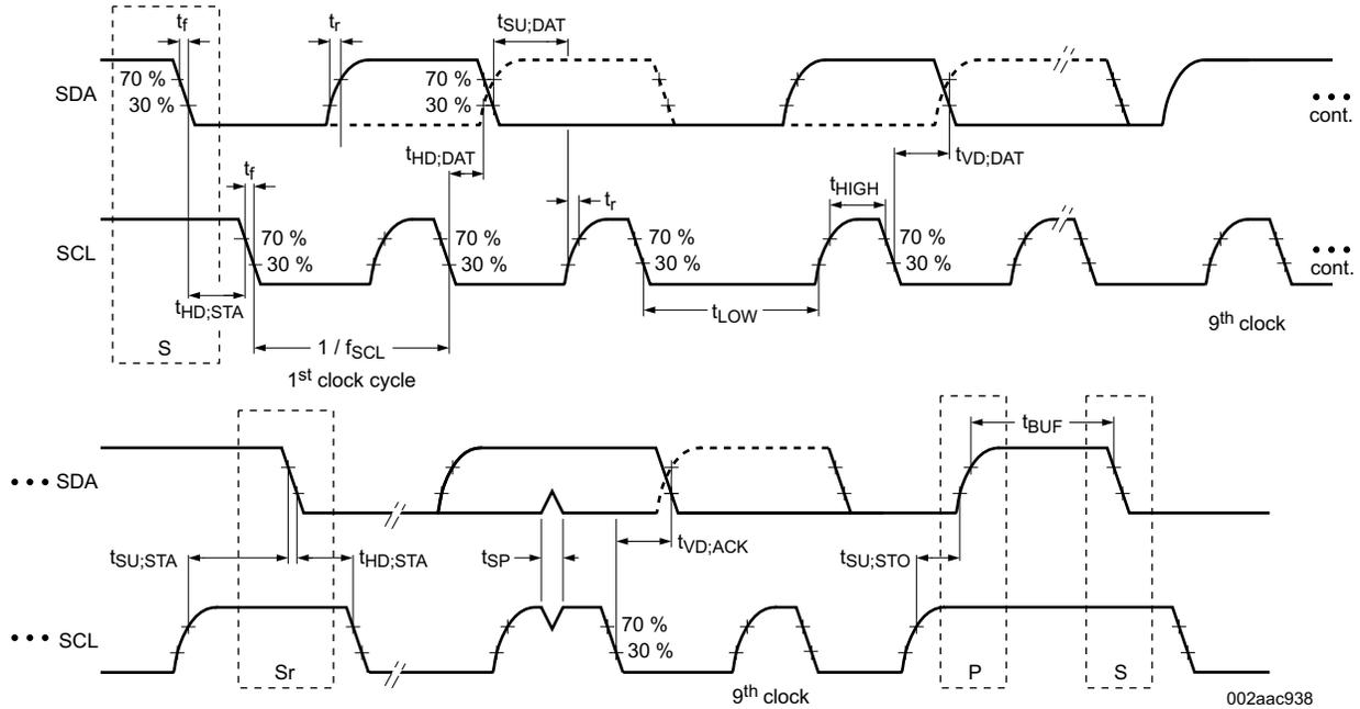
图 8-1. I<sup>2</sup>C Slave Interface Timing
