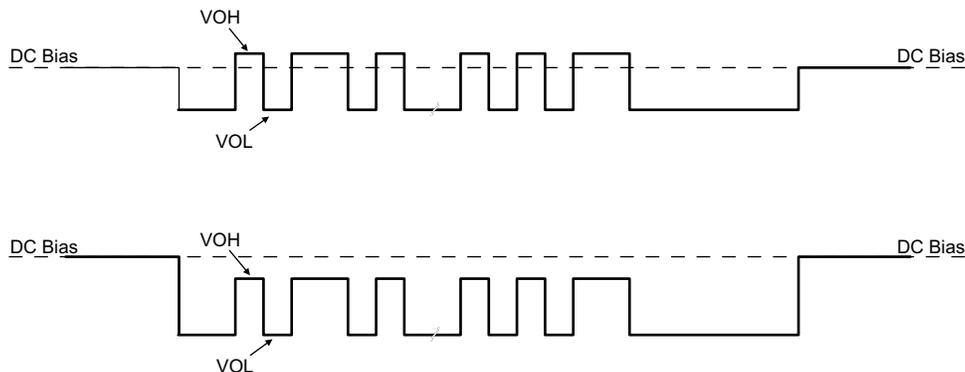
**图 9-23. TX Driver Transmission with DC Bias**
