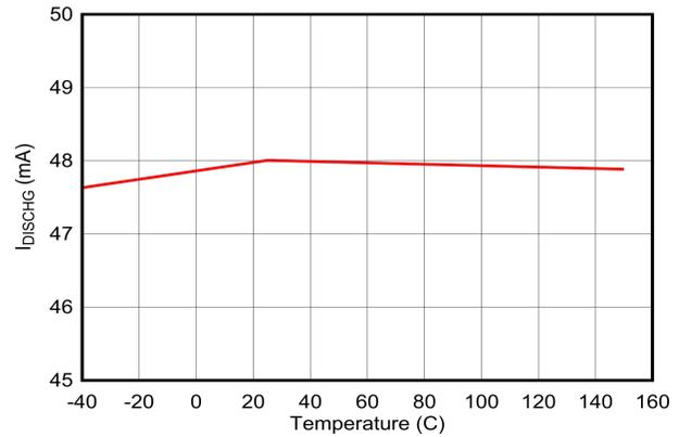
图 7-34.  $V_{BUS}$  Discharge Current vs Temperature
