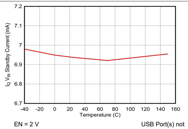
图 7-2.  $I_{Q\ V_{IN}}$  Standby Current vs Temperature
