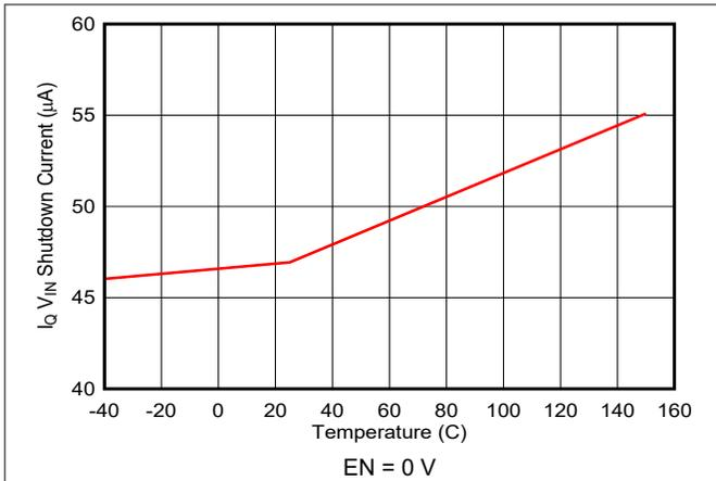
图 7-1.  $I_{Q\ V_{IN}}$  Shutdown Current vs Temperature
