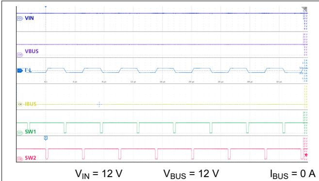
图 10-22. Buck-Boost Mode:  $V_{IN} = V_{BUS}$ , No Load
