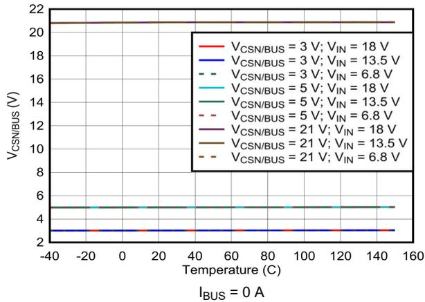
图 7-33. Buck-boost Output Voltage Regulation vs Temperature
