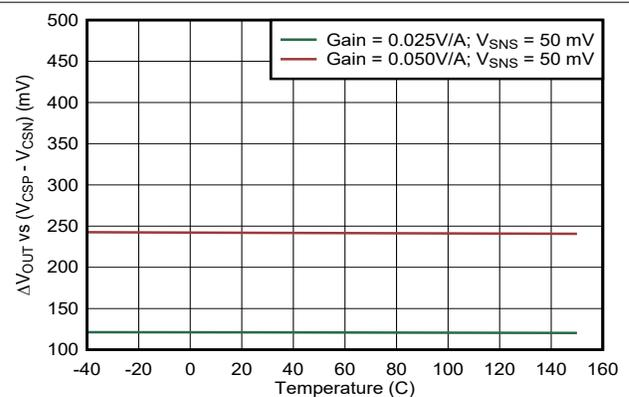
Figure 7-30. Cable Voltage Droop Compensation vs Temperature
