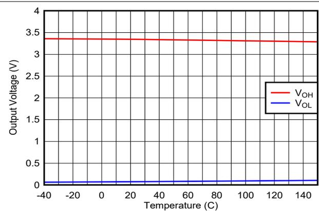
图 7-46. GPIO: Output Voltage vs Output Current and Temperature
