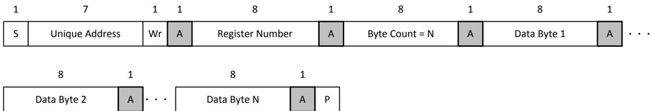
图 9-38. I<sup>2</sup>C Unique Address Write Register Protocol
