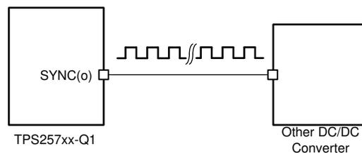
**图 9-15. Using SYNC(o) to slave DC/DC Converter**
