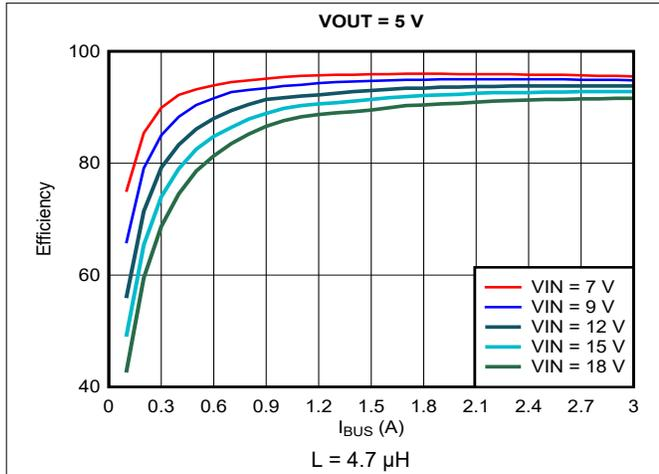
图 10-6. Efficiency vs Output Current ( $I_{OUT}$ ),  $V_{OUT} = 5\text{ V}$
