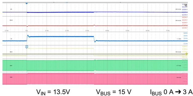
$V_{IN} = 13.5V$        $V_{BUS} = 15V$        $I_{BUS} 0A \rightarrow 3A$
