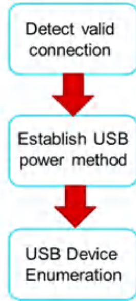
图 10-26. Flow of DFP to UFP Configuration
