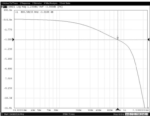
图 8-29. Data Transmission Characteristics vs Frequency (TPS25830A-Q1)
