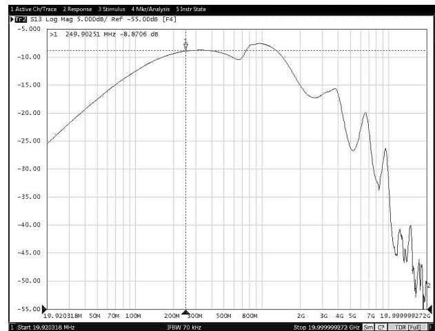
图 8-30. Off-State Data-Switch Isolation vs Frequency (TPS25830A-Q1)
