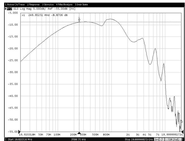
图 8-30. Off-State Data-Switch Isolation vs Frequency (TPS25830A-Q1)
