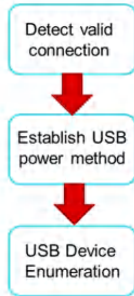
图 10-26. Flow of DFP to UFP Configuration
