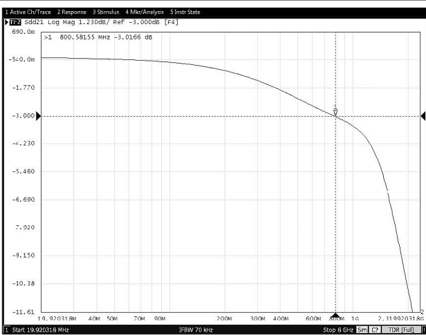
图 8-23. Data Transmission Characteristics vs Frequency
