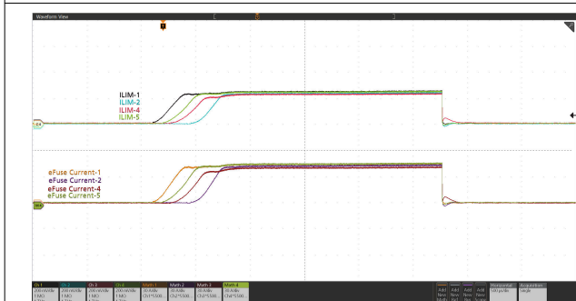
图 9-8. Power Up into Short (Current distribution among five devices in parallel): V_{IN} = 12 V, EN/UVLO Stepped Up From 0 V to 3 V, R_{IREF} = 40.2 k \Omega , R_{ILIM} on Each Device = 300 \Omega , and OUT Shorted to GND
