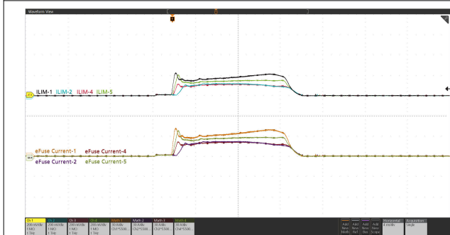
图 9-6. Start-up with EN/UVLO (Current distribution among five devices in parallel): V_{IN} = 12 V, EN/UVLO Stepped Up From 0 V to 3 V, C_{LOAD} = 55 mF, C_{DVDT} = 33 nF, R_{IREF} = 40.2 k \Omega , and R_{ILIM} on Each Device = 300 \Omega
