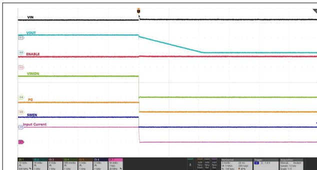
IN supply held steady at 12 V, EN pin held high, PMBus OPERATION OFF Command. C_{OUT} = 18\text{ mF} , C_{dVdt} = 33\text{ nF}
