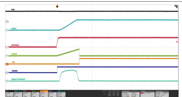
IN supply held steady at 12 V, EN pin toggled from low to high. C_{OUT} = 18\text{ mF} , C_{dVdt} = 33\text{ nF}
