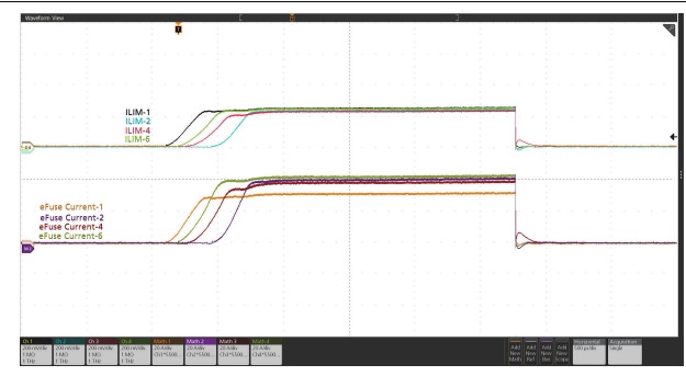
图 9-8. Power Up into Short (Current distribution among six devices in parallel): V_{IN} = 12 V, EN/UVLO Stepped Up From 0 V to 3 V, V_{IREF} = 1 V, R_{ILIM(TPS25990)} = 422 \Omega , R_{ILIM(TPS25985)} = 316 \Omega , and OUT Shorted to GND
