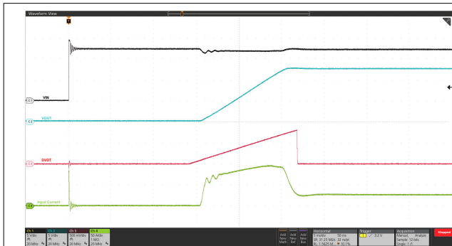
图 9-5. Input Hot Plug: V_{IN} Stepped Up from 0 V to 12 V, C_{LOAD} = 50 mF, R_{LOAD(Start-up)} = 0.48 \Omega , C_{DVDT} = 33 nF, V_{IREF} = 1 V, R_{ILIM(TPS25990)} = 422 \Omega , and R_{ILIM(TPS25985)} = 316 \Omega
