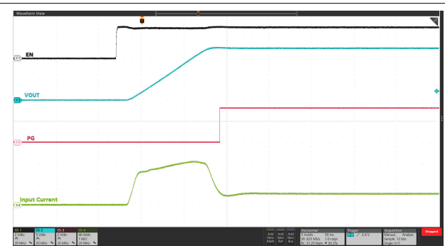
图 9-6. Start-up with EN/UVLO: V_{IN} = 12 V, EN/UVLO Stepped Up From 0 V to 3 V, C_{LOAD} = 50 mF, R_{LOAD(Start-up)} = 0.48 \Omega , C_{DVDT} = 33 nF, V_{IREF} = 1 V, R_{ILIM(TPS25990)} = 422 \Omega , and R_{ILIM(TPS25985)} = 316 \Omega
