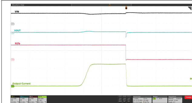
图 9-7. Power Up into Short: V_{IN} = 12 V, EN/UVLO Stepped Up From 0 V to 3 V, V_{IREF} = 1 V, R_{ILIM(TPS25990)} = 422 \Omega , R_{ILIM(TPS25985)} = 316 \Omega , and OUT Shorted to GND
