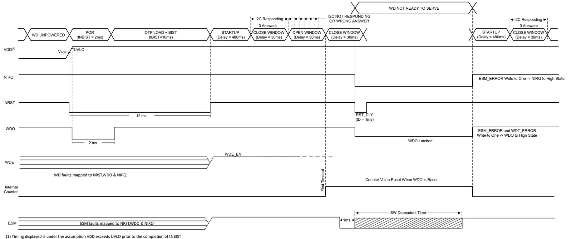
图 7-19. TPS389C03 ESM Error After WD Time-out
