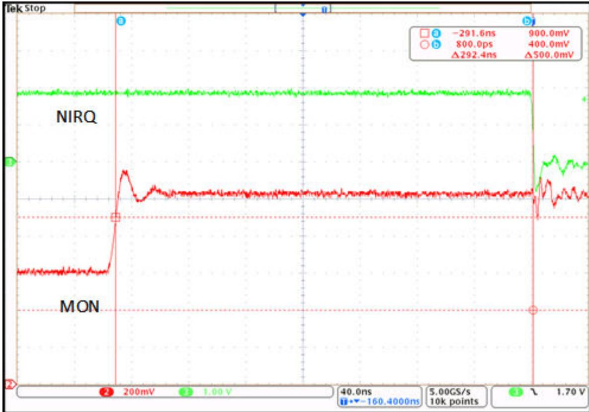
图 9-8. NIRQ Propagation Delay Resulting from Overvoltage Fault
