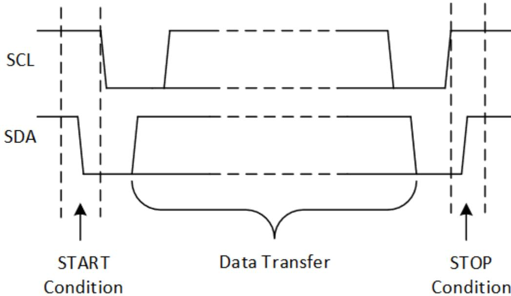
图 7-5. I<sup>2</sup>C START and STOP condition
