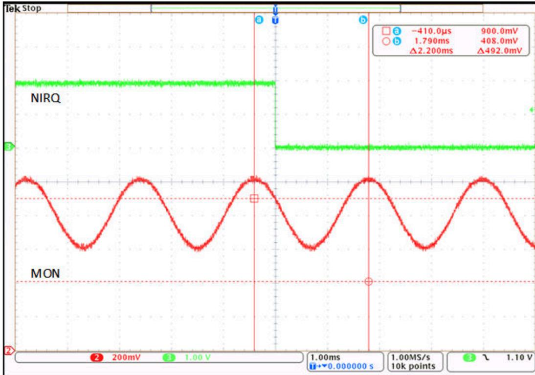
**图 9-11. 250Hz Low Pass Filter setting. NIRQ Triggered at 455Hz Signal With a 0.8V DC Component and 200mVp-p AC Signal. OV and UV Thresholds Set to 0.9V and 0.7V. Reduced the Frequency From 500Hz Until the NIRQ Pin Went Low.**
