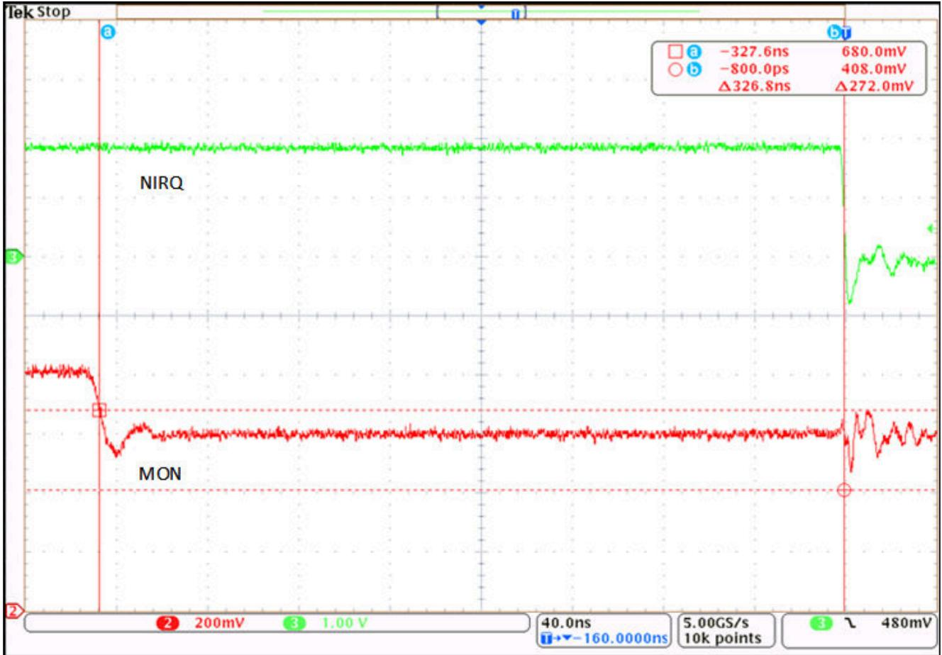
图 9-9. NIRQ Propogation Delay Resulting from Undervoltage Fault
