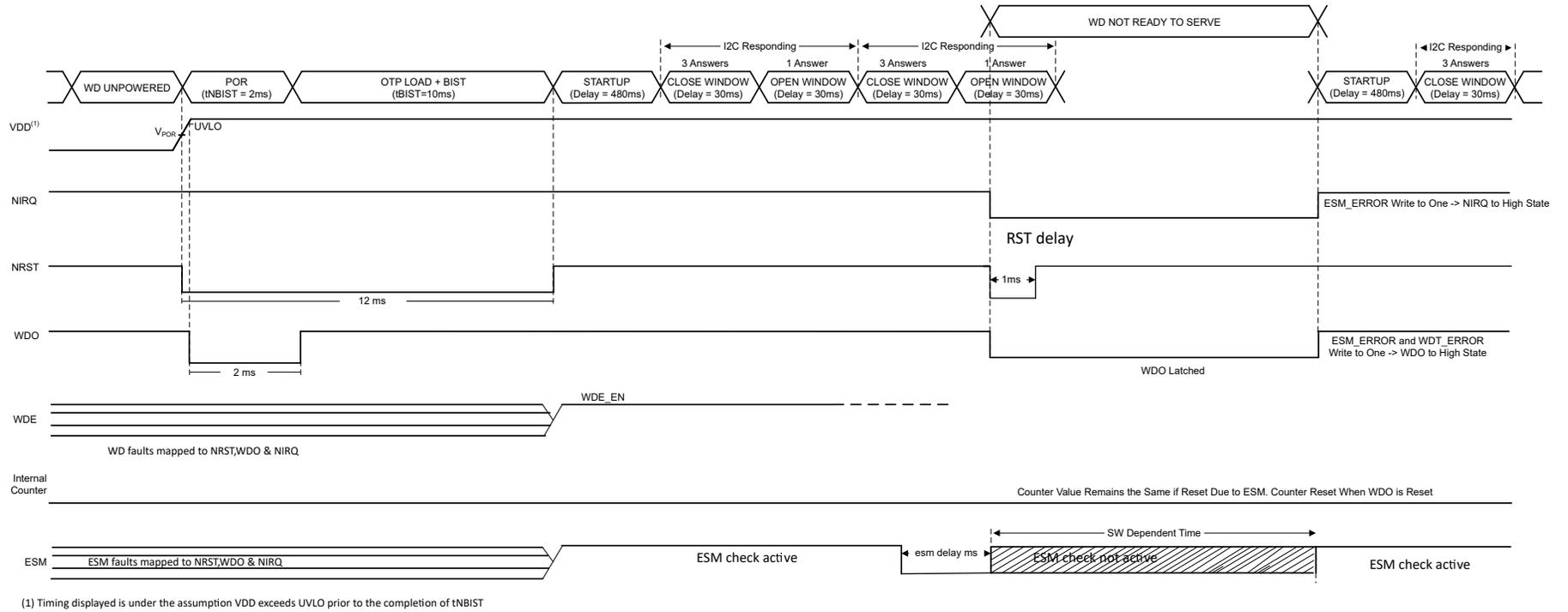
图 7-27. ESM Fault (WD Enabled)
