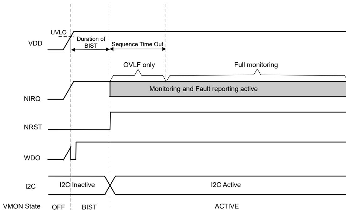
**图 7-31. TPS389C03-Q1 Power ON Signaling and Internal States**
