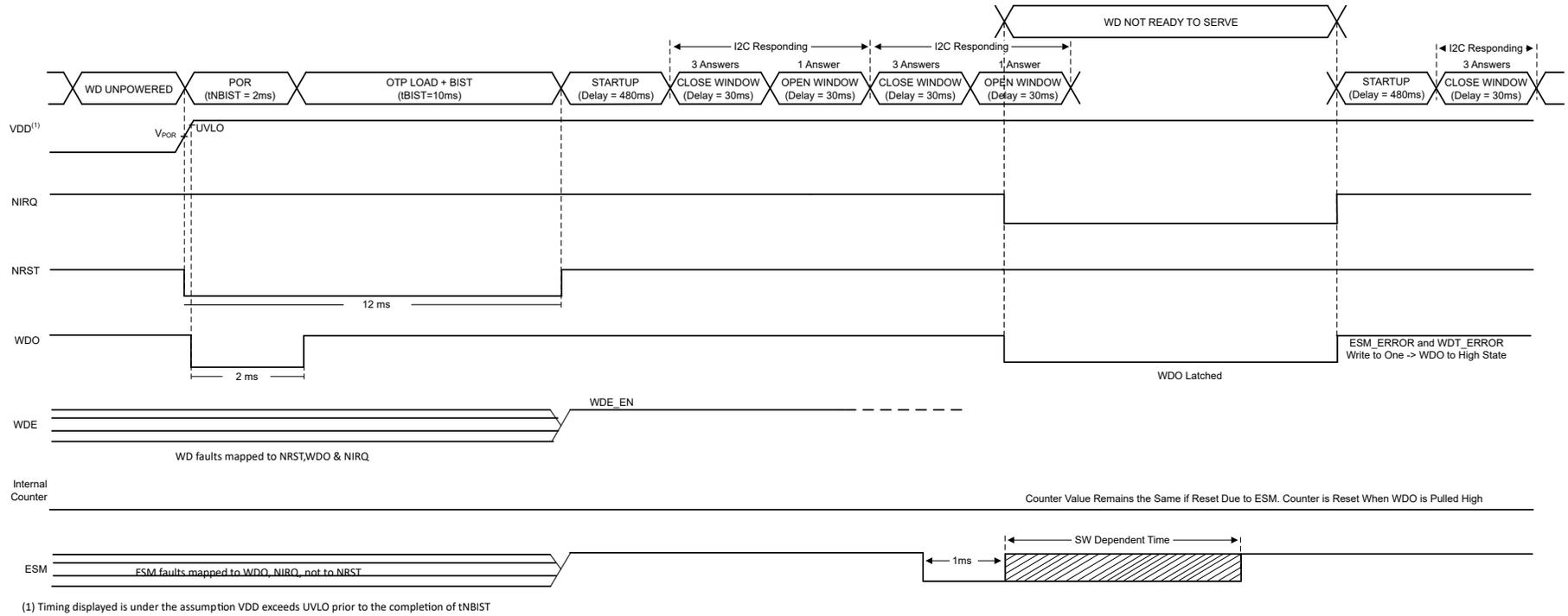
**图 7-18. TPS389C03 ESM Error with No WD Faults**
