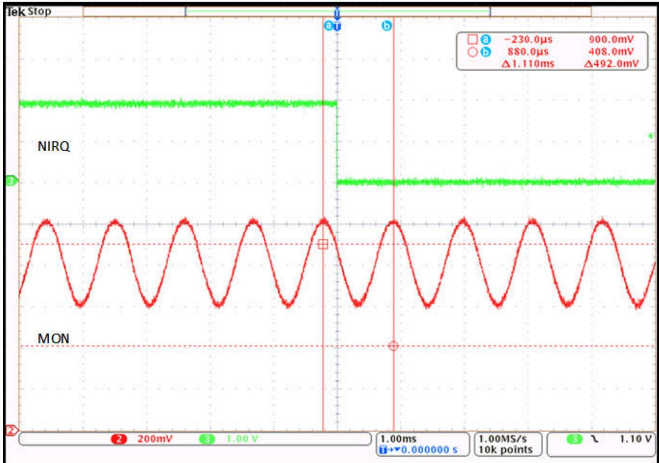
图 9-12. 500Hz Low Pass Filter Setting. NIRQ Triggered at 0.9kHz Signal With a 0.8V DC Component and 200mVp-p AC Signal. OV and UV Thresholds Set to 0.9V and 0.7V. Reduced the Frequency From 1kHz Until the NIRQ Pin Went Low.
