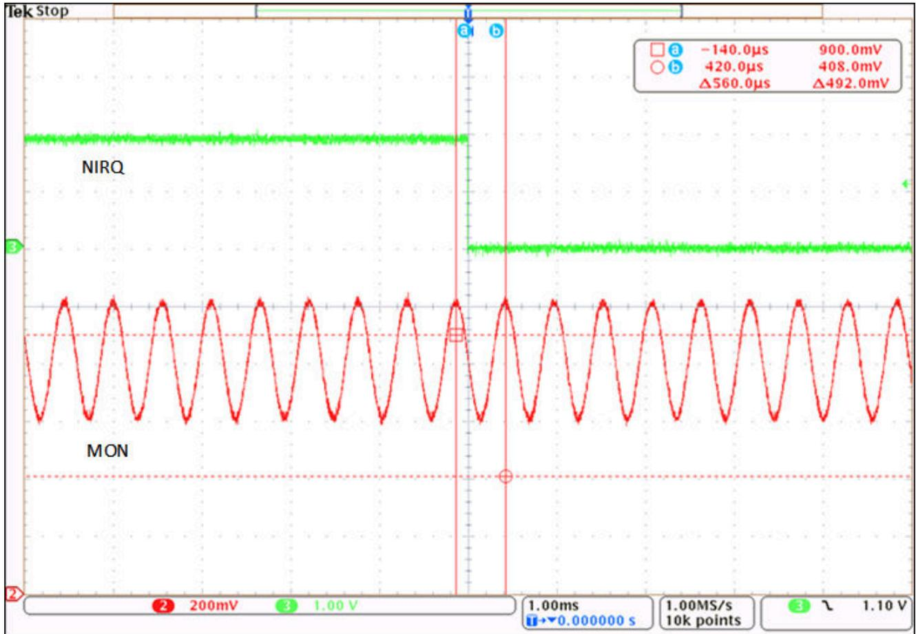
图 9-10. 1kHz Low Pass Filter Setting. NIRQ Triggered at 1.8kHz Signal with a 0.8V DC Component and 200mVp-p AC Signal. OV and UV Thresholds Set to 0.9V and 0.7V. Reduced the Frequency From 2kHz Until the NIRQ Pin Went Low.
