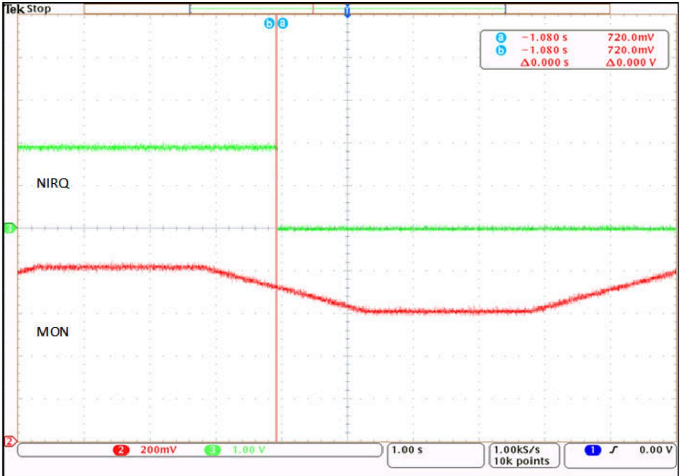
图 9-3. NIRQ Triggered After an Undervoltage Fault
