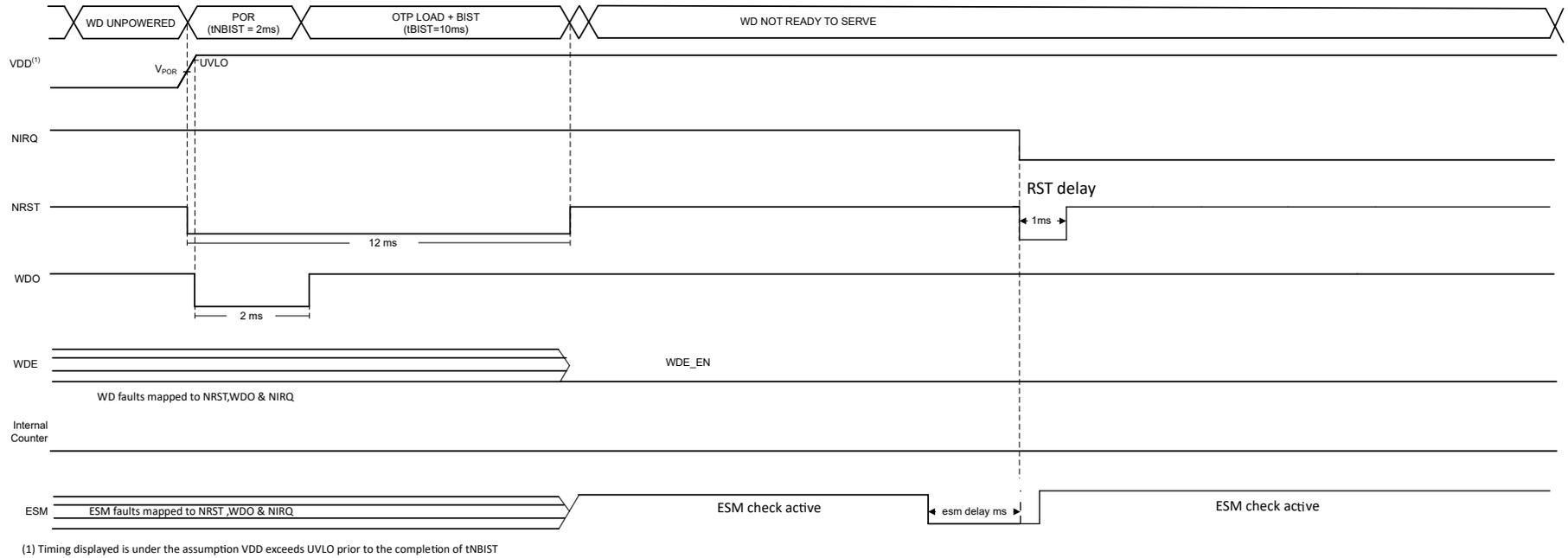
图 7-28. Transient ESM Fault (WD Disabled)
