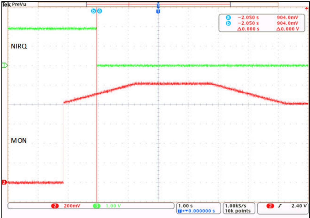
图 9-2. NIRQ Triggered After an Overvoltage Fault
