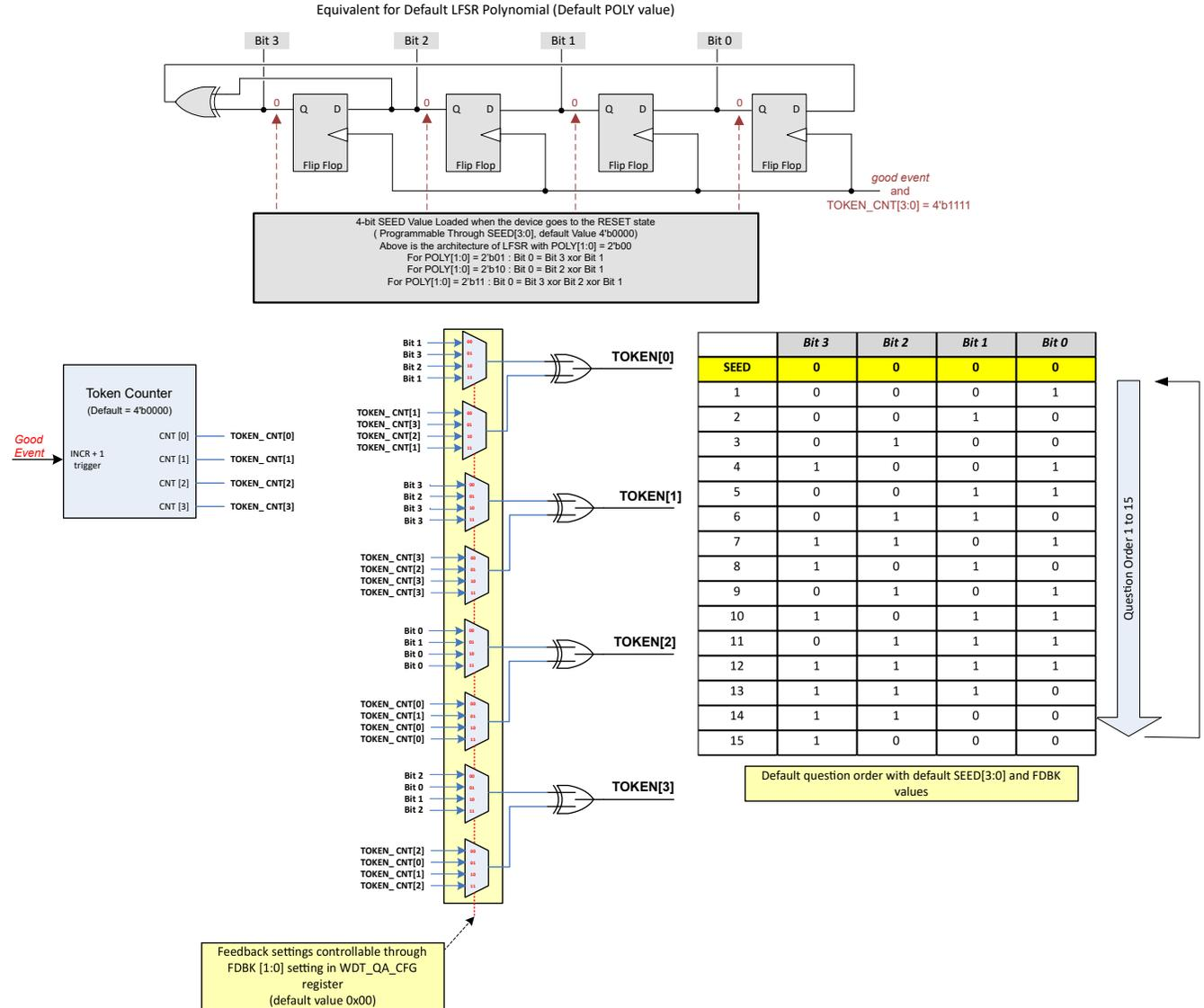
A. A value of 0000b is a special seed and equates to 0001b, including the default loading of 0000b during power up.
