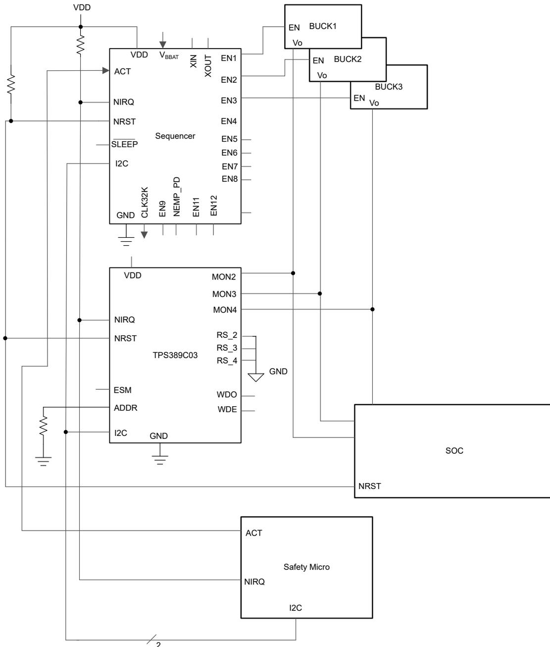
图 9-1. TPS389C03-Q1 Voltage Monitor Design Block Diagram
