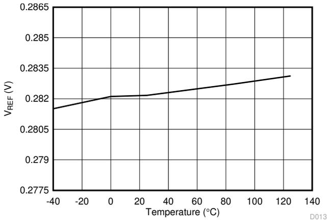
**图 6-13. Reference Voltage vs Temperature ( $V_{REF} = 0.282\text{ V}$ )**
