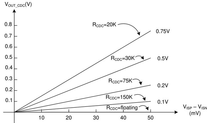
图 7-6. Output Voltage Rise vs Output Current
