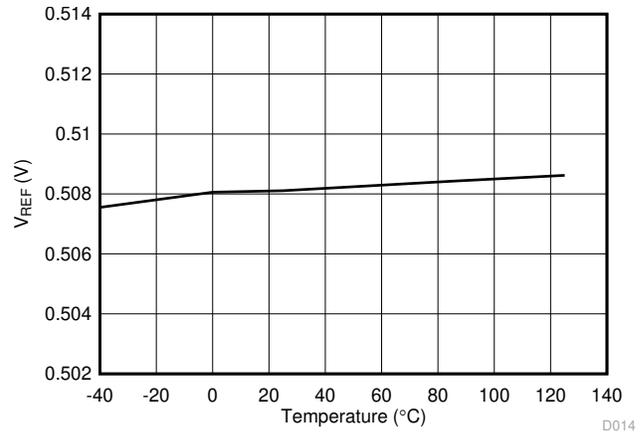
**图 6-14. Reference Voltage vs Temperature ( $V_{REF} = 0.508\text{ V}$ )**
