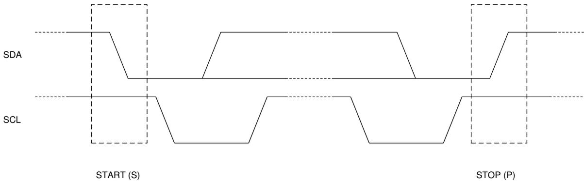
图 7-8. I<sup>2</sup>C START and STOP Conditions
