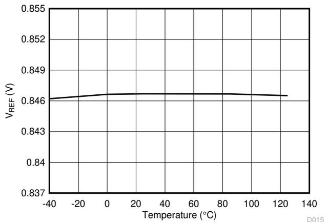
**图 6-15. Reference Voltage vs Temperature ( $V_{REF} = 0.846\text{ V}$ )**
