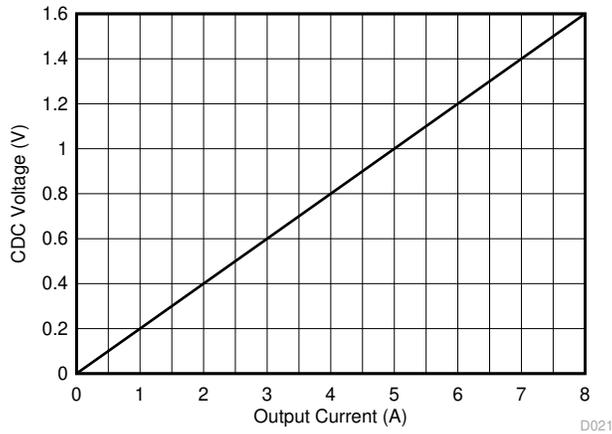
图 6-21. CDC Voltage vs Output Current with R<sub>SENSE</sub> = 10 mΩ
