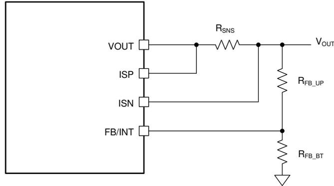
图 7-5. Output Voltage Setting by External Resistor Divider
