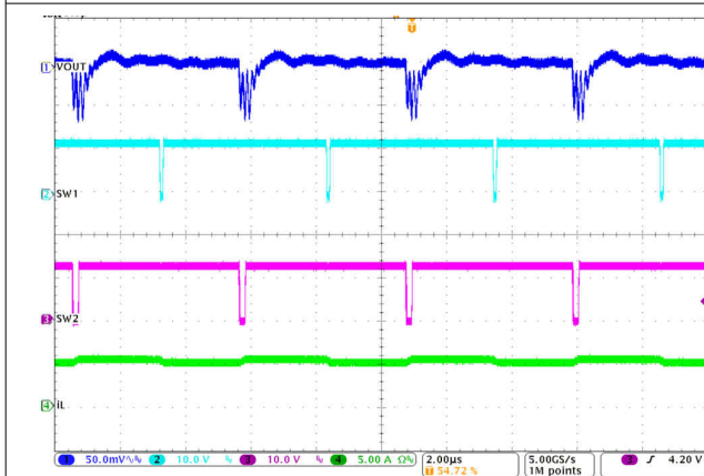
图 8-4. Switching Waveforms in V_{IN} = 12\text{ V} , V_{OUT} = 12\text{ V} , I_O = 5\text{ A} , FPWM
