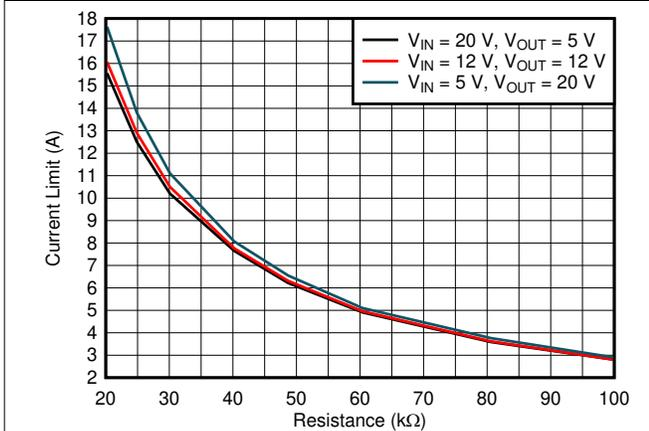
图 6-11. Average Inductor Current Limit vs Setting Resistance
