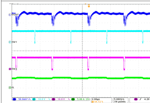
图 8-4. Switching Waveforms in V_{IN} = 12\text{ V} , V_{OUT} = 12\text{ V} , I_O = 5\text{ A} , FPWM
