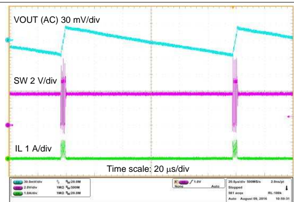
V_{OUT} = 5\text{ V} , V_{IN} = 3.6\text{ V} , I_{OUT} = 10\text{ mA} , T_A = 25\text{ }^\circ\text{C}
