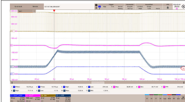
V_{IN} = 5.0V BOM = 4 \times 22 \mu F V_{OUT} = 1.2V I_{OUT} = 10mA \text{ 至 } 10A, 1A/\mu s 图 9-30. 负载瞬态 - FPWM 运行
