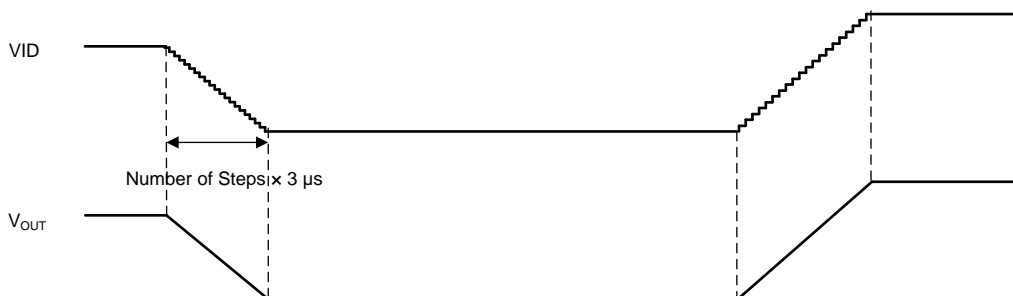
Figure 5-5. DVS Timing Diagram I (BUCKx_DECAY = 0)
