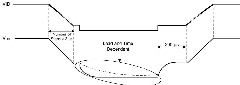
图 6-5. DVS Timing Diagram II (BUCKx\_DECAY = 0b)
