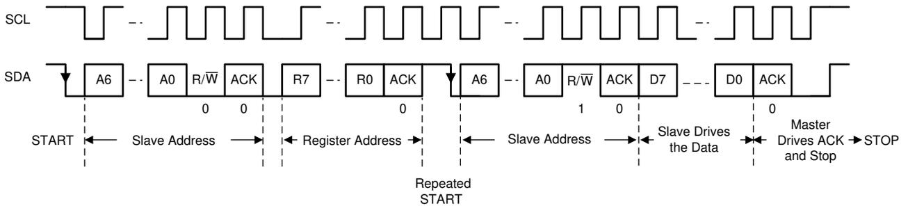
图 6-14. I<sup>2</sup>C Interface READ From TPS6508700 in F/S Mode (Only Repeated START is Supported)
