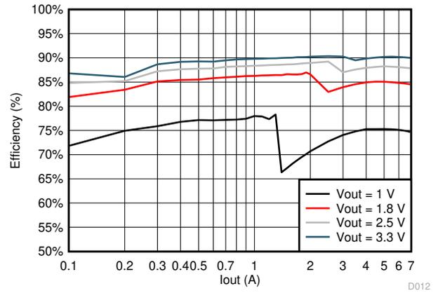
图 5-4. BUCK6 Efficiency at  $V_{IN} = 18V$
