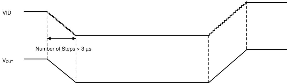
图 6-4. DVS Timing Diagram I (BUCKx\_DECAY = 0b)
