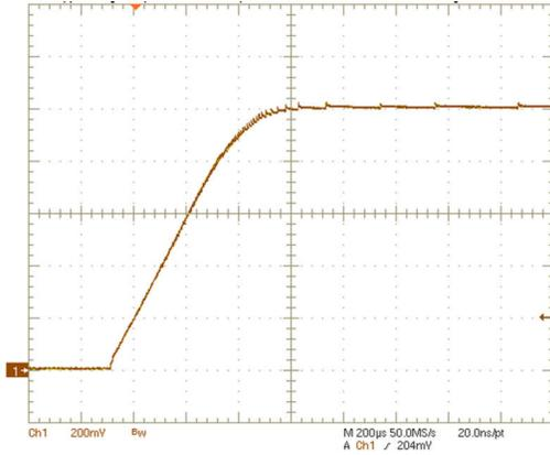
图 5-1. BUCK2 Controller Start Up to 1V by I<sup>2</sup>C
