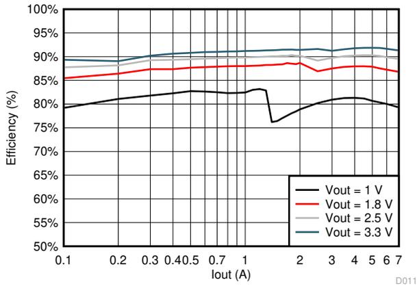
图 5-3. BUCK6 Efficiency at  $V_{IN} = 13V$
