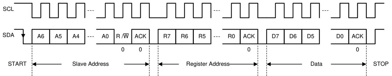
图 6-13. I<sup>2</sup>C Interface WRITE to TPS6508700 in F/S Mode
