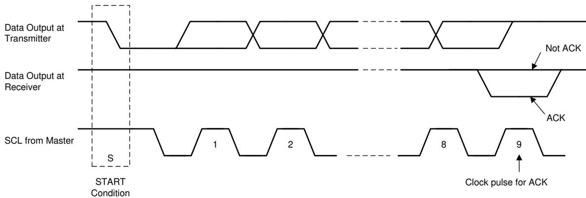
图 6-11. Acknowledge on the I<sup>2</sup>C Bus
