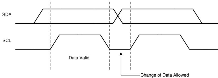
图 6-10. Bit Transfer on the I<sup>2</sup>C Bus
