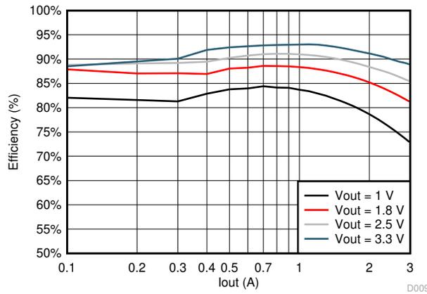
图 5-5. Converter Efficiency at  $V_{IN} = 5V$
