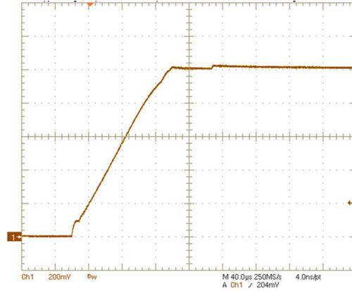
图 5-2. Converter Start Up to 1V by I<sup>2</sup>C
