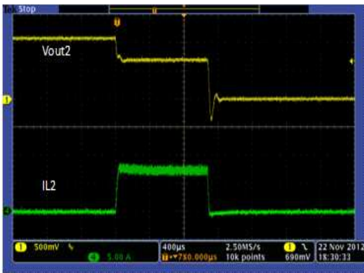
Figure 29. Over Current Protection, Buck 2
