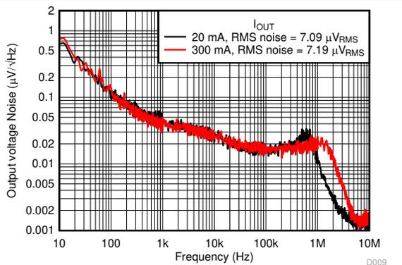
图 5-71. Noise vs Frequency and  $I_{OUT}$
