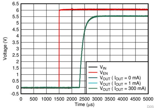
$V_{OUT} = 5.5\text{ V}$ ,  $V_{IN} = 0\text{ V}$  to  $6.0\text{ V}$ ,  $V_{EN} = 0\text{ V}$  to  $6.0\text{ V}$ ,  $V_{EN}$  rises  $500\text{ }\mu\text{s}$  ahead of  $V_{IN}$ ,  $V_{IN}$  and  $V_{EN}$  slew rate =  $1\text{ V}/\mu\text{s}$
