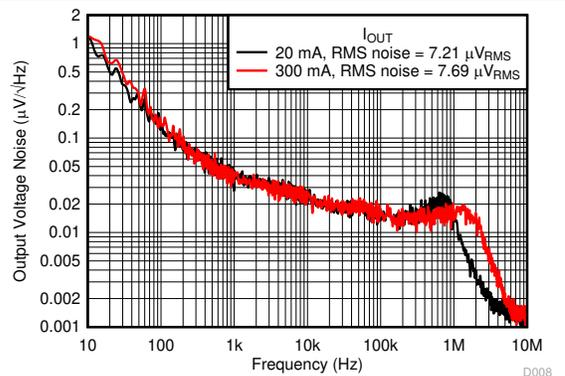
图 5-72. Noise vs Frequency and  $I_{OUT}$
