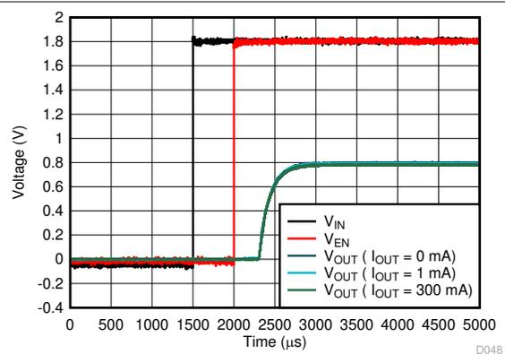
$V_{OUT} = 0.8\text{ V}$ ,  $V_{IN} = 0\text{ V}$  to  $1.8\text{ V}$ ,  $V_{EN} = 0\text{ V}$  to  $1.8\text{ V}$ ,  $V_{EN}$  rises  $500\text{ }\mu\text{s}$  behind  $V_{IN}$ ,  $V_{IN}$  and  $V_{EN}$  slew rate =  $1\text{ V}/\mu\text{s}$
