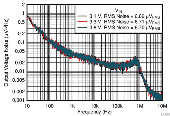
$I_{OUT} = 20\text{ mA}, V_{RMS}\text{ BW} = 10\text{ Hz to }100\text{ kHz}$
