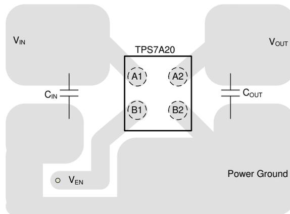
图 7-9. YCJ and YCK Package (DSBGA) Typical Layout
