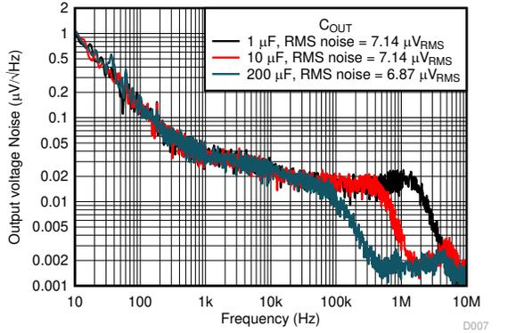
图 5-69. Noise vs Frequency and  $C_{OUT}$
