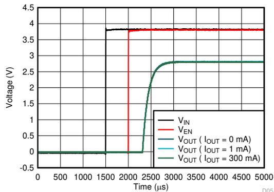
$V_{IN} = 0\text{ V}$  to  $3.8\text{ V}$ ,  $V_{EN} = 0\text{ V}$  to  $3.8\text{ V}$ ,  $V_{EN}$  rises  $500\text{ }\mu\text{s}$  behind  $V_{IN}$ ,  $V_{IN}$  and  $V_{EN}$  slew rate =  $1\text{ V}/\mu\text{s}$
