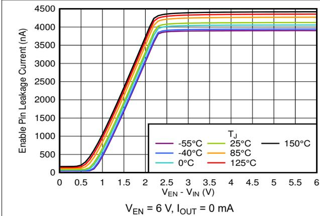
图 5-43. Enable Pin Leakage Current vs  $V_{EN} - V_{IN}$
