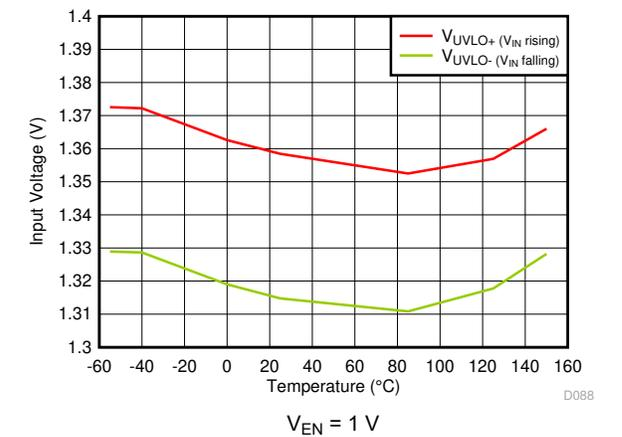
图 5-46. UVLO Threshold vs Temperature
