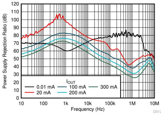
图 5-63. PSRR vs Frequency and  $I_{OUT}$
