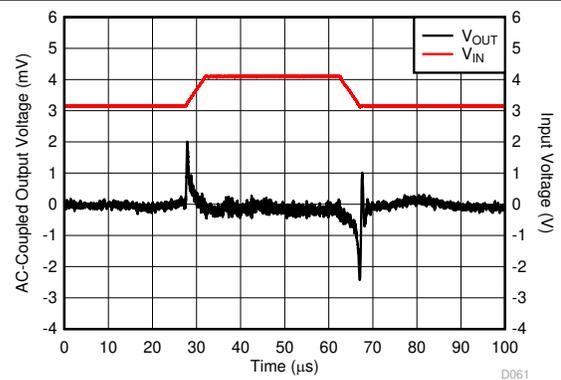
$V_{IN} = 3.1\text{ V} \rightarrow 4.1\text{ V} \rightarrow 3.1\text{ V}$ ,  $V_{IN} t_{RISING} = 5\text{ }\mu\text{s}$ ,
