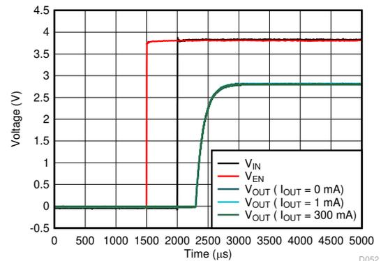
$V_{IN} = 0\text{ V}$  to  $3.8\text{ V}$ ,  $V_{EN} = 0\text{ V}$  to  $3.8\text{ V}$ ,  $V_{EN}$  rises  $500\text{ }\mu\text{s}$  ahead of  $V_{IN}$ ,  $V_{IN}$  and  $V_{EN}$  slew rate =  $1\text{ V}/\mu\text{s}$
