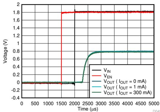
$V_{OUT} = 0.8\text{ V}$ ,  $V_{IN} = 0\text{ V}$  to  $1.8\text{ V}$ ,  $V_{EN} = 0\text{ V}$  to  $1.8\text{ V}$ ,  $V_{EN}$  rises  $500\text{ }\mu\text{s}$  ahead of  $V_{IN}$ ,  $V_{IN}$  and  $V_{EN}$  slew rate =  $1\text{ V}/\mu\text{s}$
