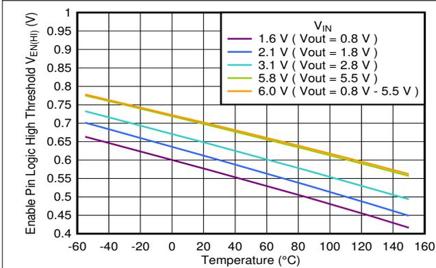
图 5-47. Enable Logic High Threshold vs Temperature
