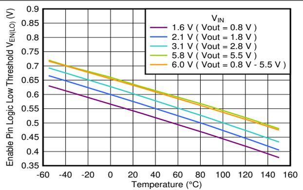
图 5-48. Enable Logic Low Threshold vs Temperature
