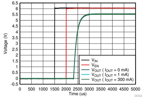
$V_{OUT} = 5.5\text{ V}$ ,  $V_{IN} = 0\text{ V}$  to  $6.0\text{ V}$ ,  $V_{EN} = 0\text{ V}$  to  $6.0\text{ V}$ ,  $V_{EN}$  rises  $500\text{ }\mu\text{s}$  behind  $V_{IN}$ ,  $V_{IN}$  and  $V_{EN}$  slew rate =  $1\text{ V}/\mu\text{s}$
