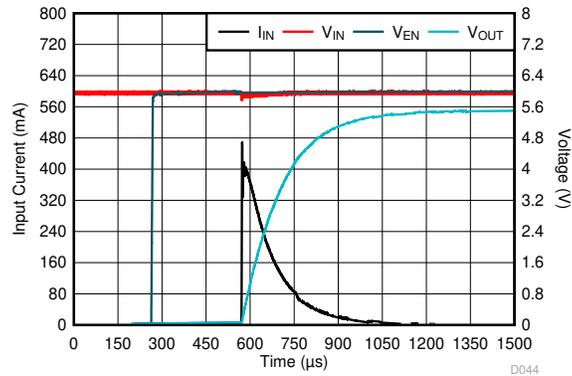
$V_{OUT} = 5.5\text{ V}$ ,  $V_{IN} = 6.0\text{ V}$ ,  $V_{EN} = 0\text{ V to }6.0\text{ V}$ ,
