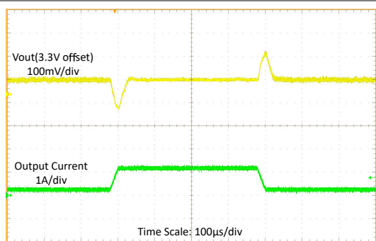
V_{IN} = 3.6V , V_{OUT} = 3.3V I_{OUT} = 100mA 至 1A , 20\mu s 压摆率
