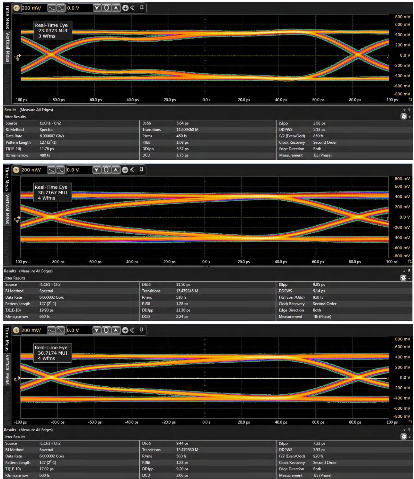
图 6-6. Typical eye diagrams at 6.0 Gbps. Top: baseline calibration setup. Middle: through TS3DV642-Q1 Port A. Bottom: through TS3DV642-Q1 Port B.
