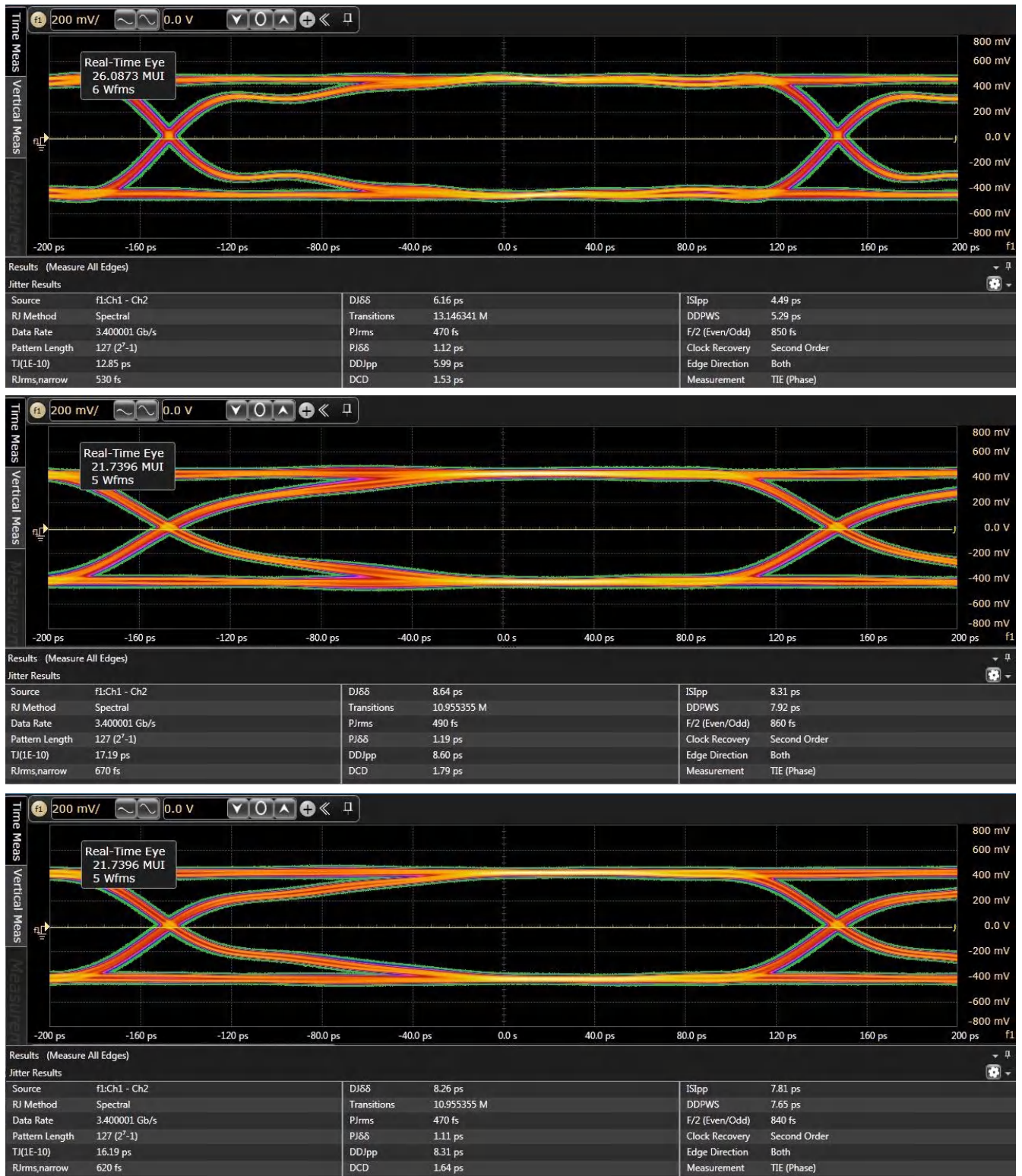
图 6-5. Typical eye diagrams at 3.4 Gbps. Top: baseline calibration setup. Middle: through TS3DV642-Q1 Port A. Bottom: through TS3DV642-Q1 Port B.
