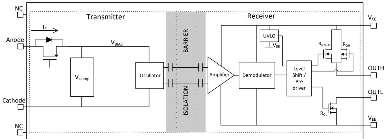
图 8-3. Functional Block Diagram for UCC23514S (Split output)
