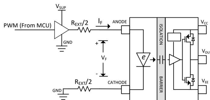
$$R_{EXT} = \frac{V_{SUP} - V_F}{I_F} - R_{OH\_buf}$$
