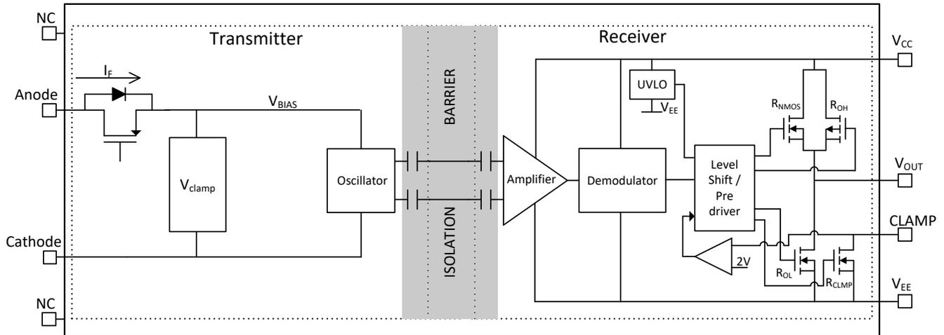
图 8-2. Functional Block Diagram for UCC23514M (Miller clamp)
