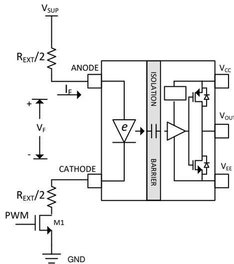
$$R_{EXT} = \frac{V_{SUP} - V_F}{I_F} - R_{M1}$$
