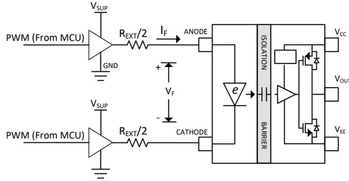
$$R_{EXT} = \frac{V_{SUP} - V_F}{I_F} - (R_{OH\_buf} + R_{OL\_buf})$$
