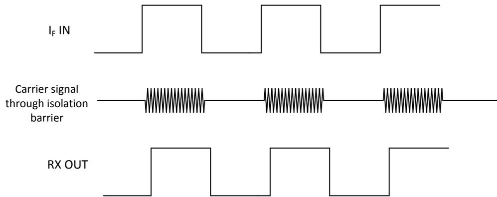
图 8-5. On-Off Keying (OOK) Based Modulation Scheme
