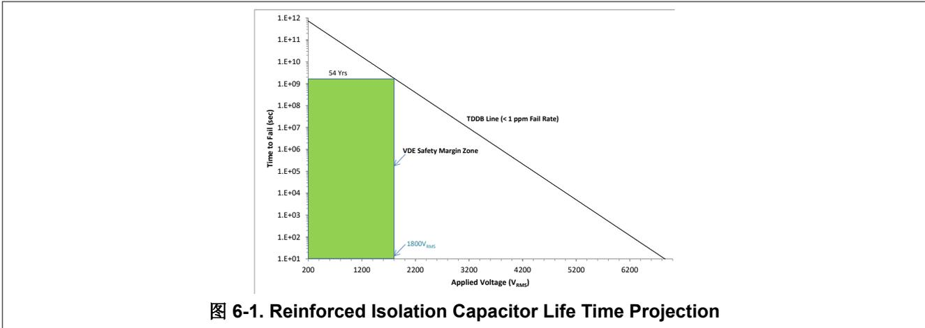
图 6-1. Reinforced Isolation Capacitor Life Time Projection
