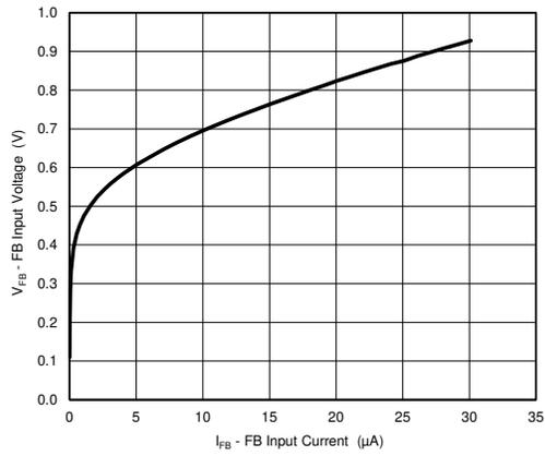
图 6-9. FB Input Voltage vs. FB Input Current
