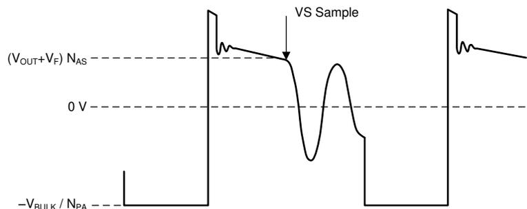
图 7-3. Auxiliary-Winding Voltage
