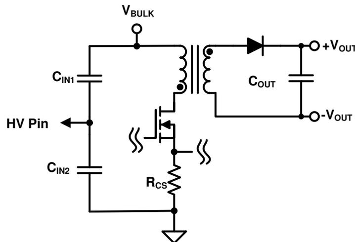
图 8-1. Implementation to Support > 700 V Inputs
