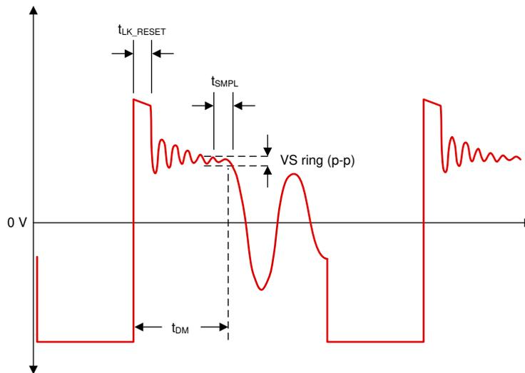
**图 7-4. Auxiliary-Winding Waveform Details**
