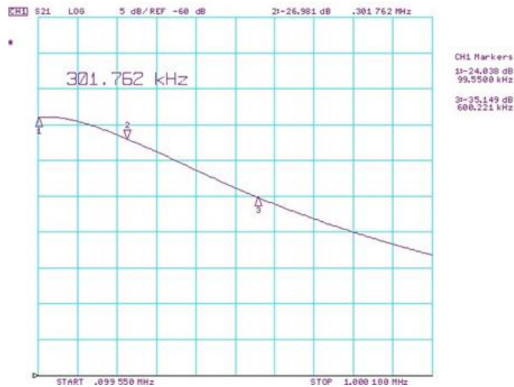
Figure 7. S21 for Modified MFB Filter Using TL081
