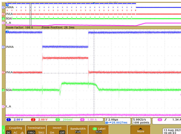
图 9-6. Driver PWM operation with feedback
