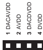
Figure 3–6. Jumper Block J3 on the DAC1220EVM
