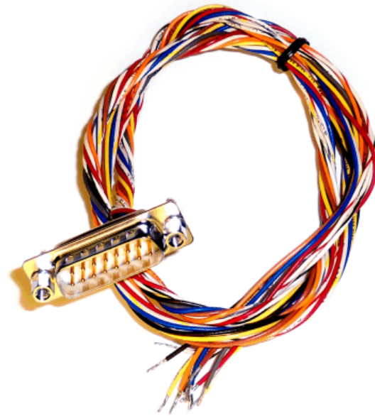
Figure 50. 15-Pin, Twisted Wire Cable
