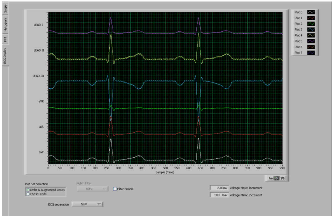
Figure 34. Normal Electrode ECG Connection in ECG Display Tab
