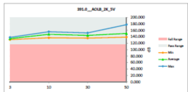
Figure 3. Radiation Exposure Effect on A_{OL} Open-Loop Voltage Gain
