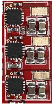
Figure 6-1. 3 Parallel TPS7A57 LDO's. The Parallel Circuitry is Boxed in White.
