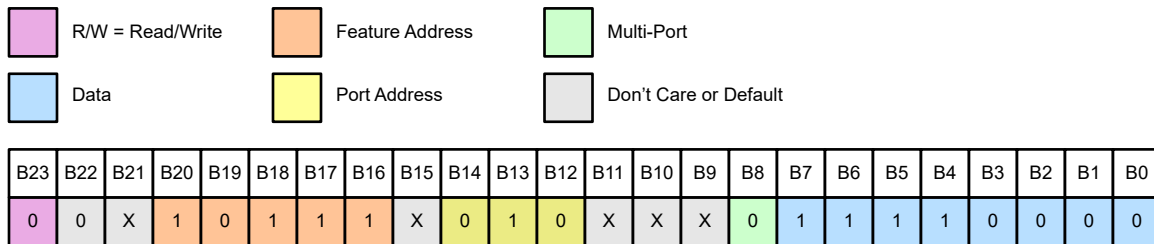
Figure 3-2. Example Write Condition (B23 = 0) to Fail-Safe Output Register 2 (B20-B16 = 0b10111), Port 2 (B14-B12 = 0b010), Multi-port disabled (B8 = 0), Set P2.7-P2.4 HIGH (B7-B4 = 0b1111), Set P2.3-P2.0 LOW (B3-B0 = 0b0000)
