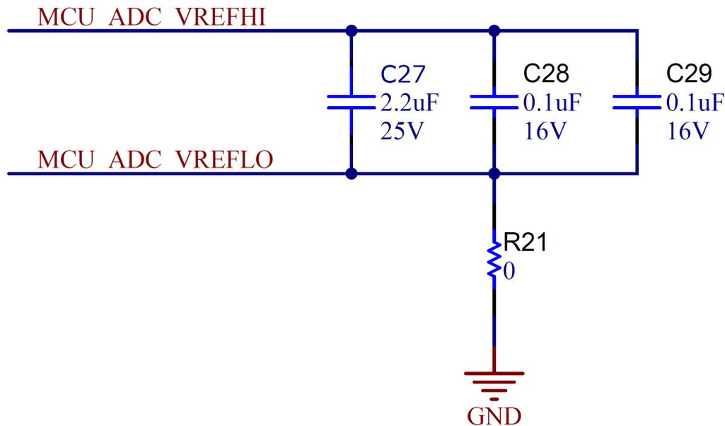
**Figure 2-10. AM13E230x VREF Decoupling Schematic**
