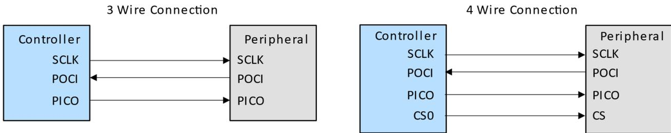
**Figure 2-3. Typical SPI Connections**
