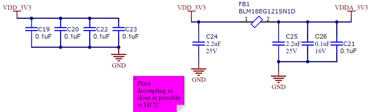
Figure 2-7. LP-AM13E230 Power Decoupling Schematic
