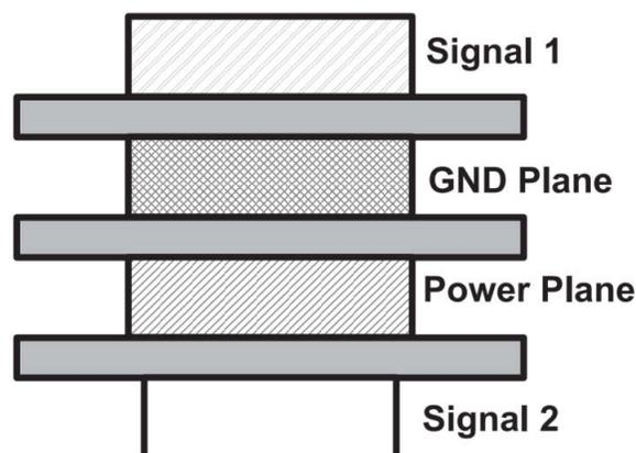
Figure 3-1. 4-Layer PCB Stack-Up
