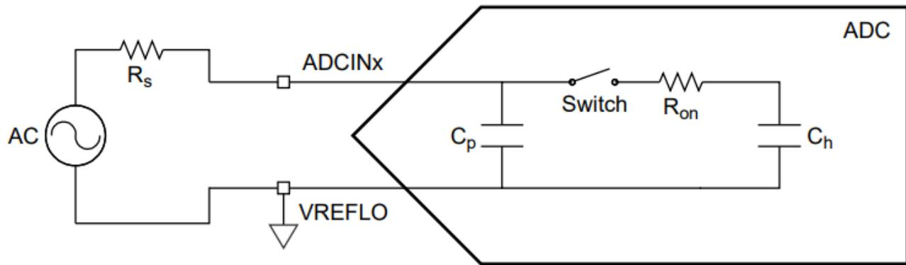
Figure 2-5. ADC Input Model
