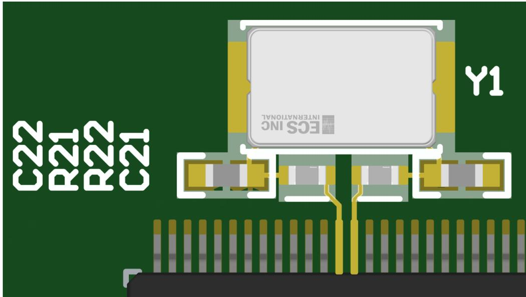
Figure 2-17. AM13E230x controlSOM Crystal Circuit - 3D View
