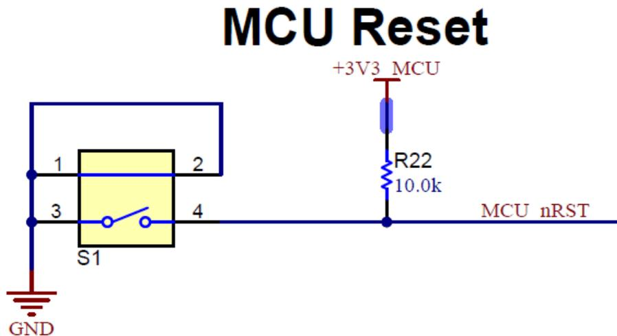
**Figure 2-13. LP-AM13E230 nRST Circuit**
