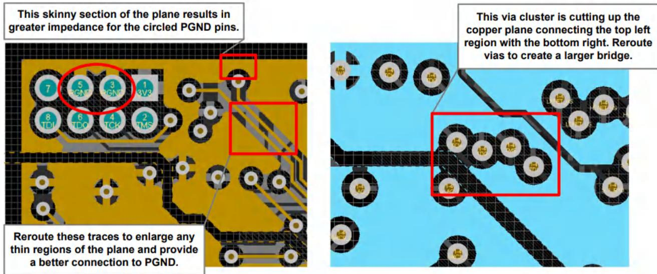
**Figure 3-7. Cut-Up GND Plane Examples**
