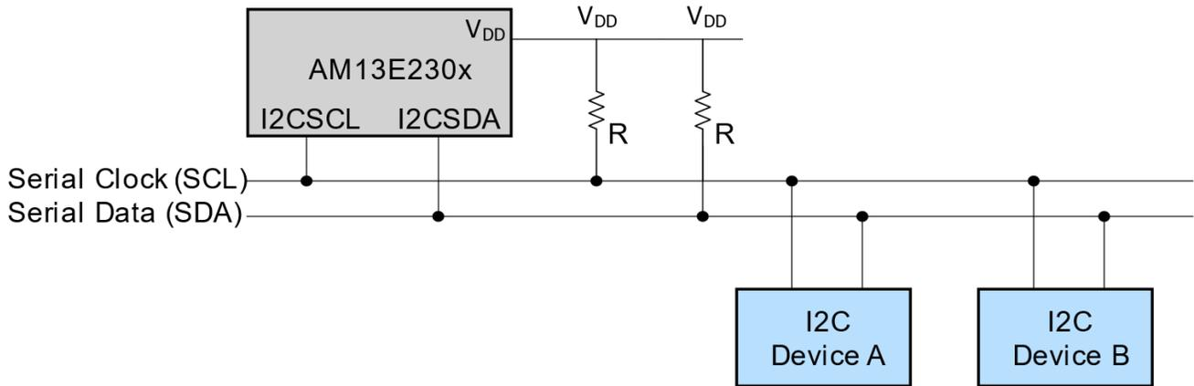
**Figure 2-2. Typical I2C Bus Connection**
