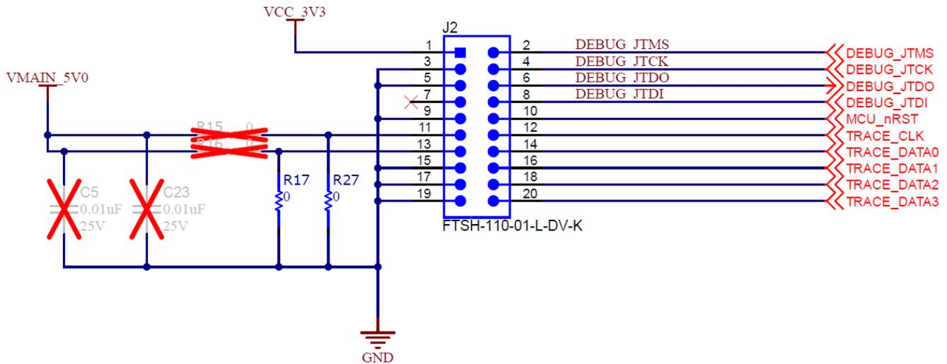
Figure 2-21. AM13E230x controlSOM Debug Header
