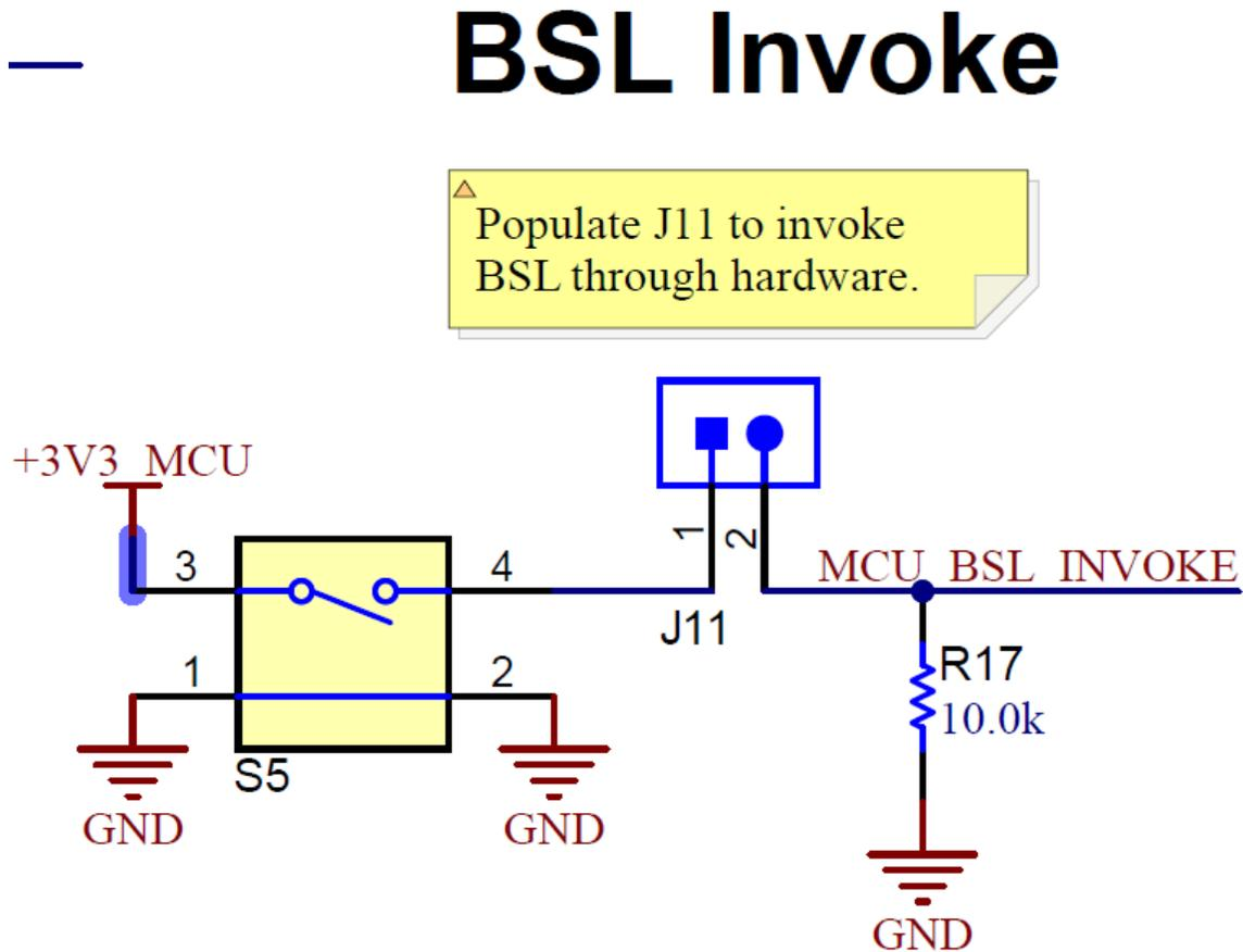
Figure 2-14. BSL Invoke Circuit
