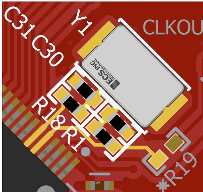
Figure 2-19. AM13E230x LaunchPad Crystal Circuit - 3D View
