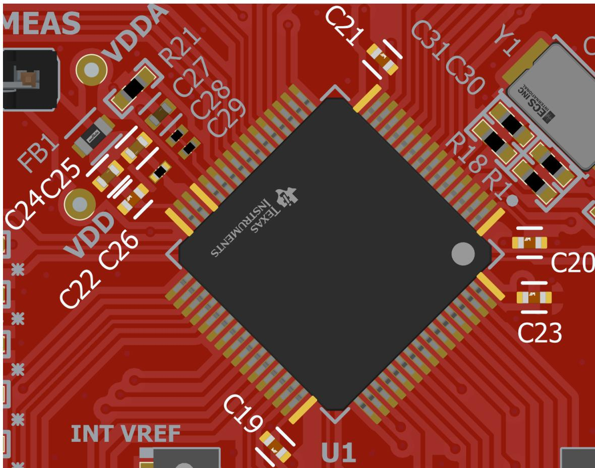
Figure 2-9. LP-AM13E230 Power Decoupling Placement – 3D View
