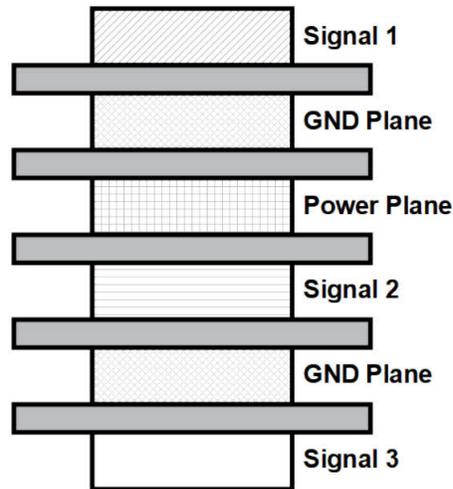
**Figure 3-3. 6-Layer PCB Stackup**
