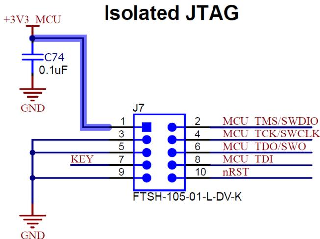
**Figure 2-20. LP-AM13E230 Debug Header**
