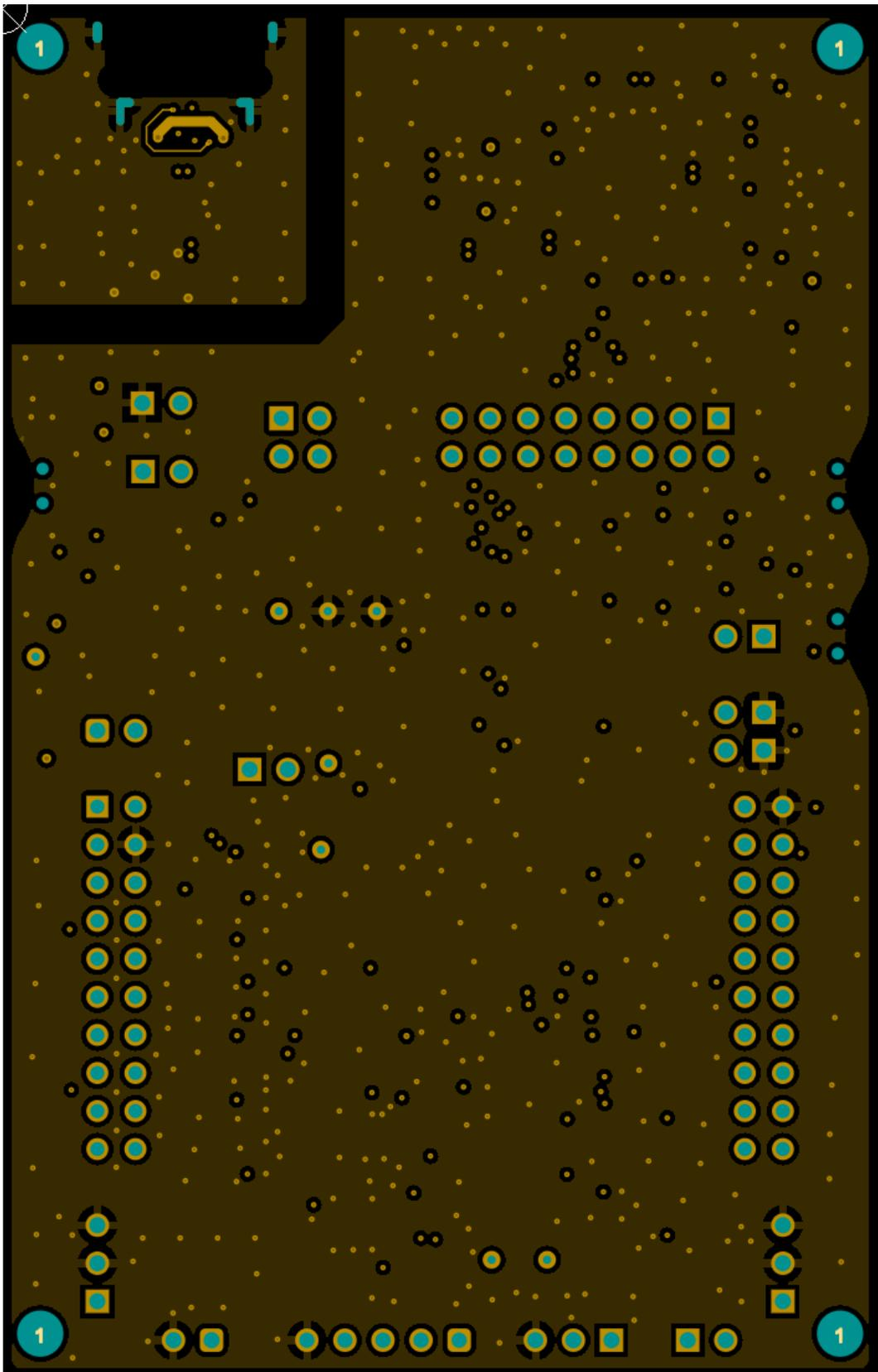
Figure 3-6. GND Plane on AM13E230x LaunchPad
