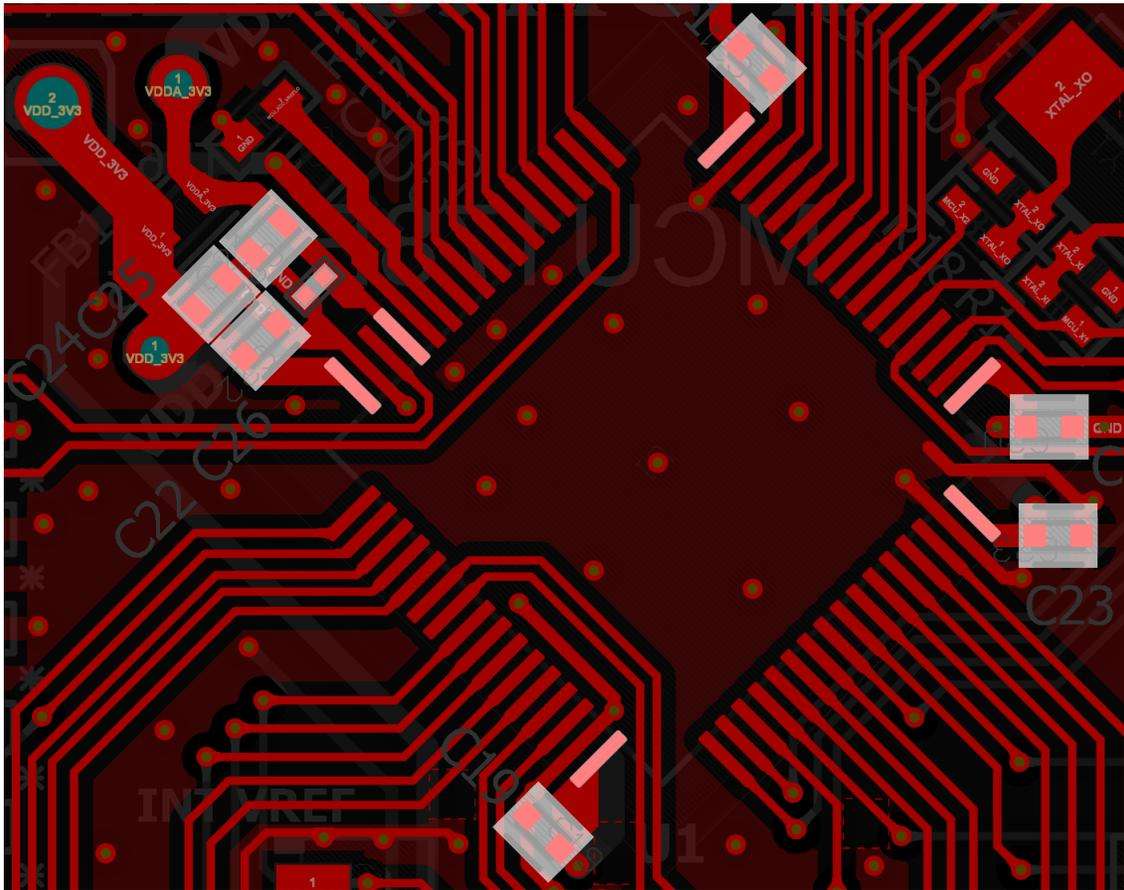
Figure 2-8. LP-AM13E230 Power Decoupling - Top Layer
