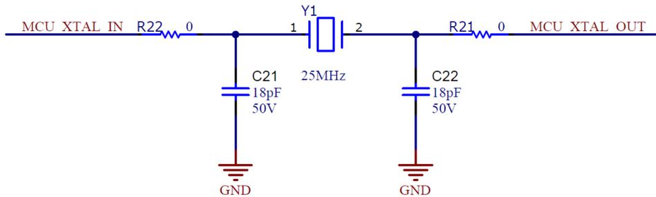
Figure 2-15. AM13E230x XTAL Circuit
