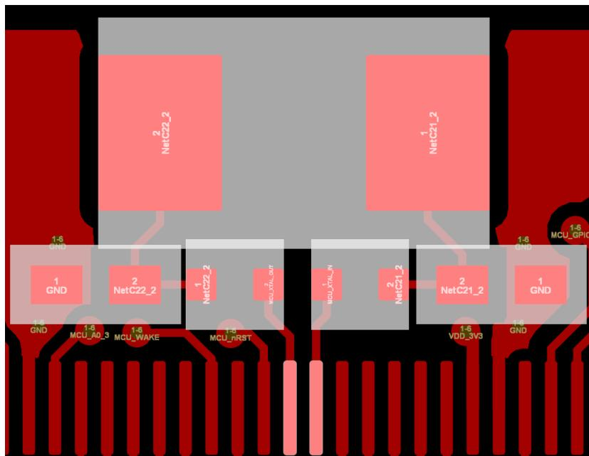
Figure 2-16. AM13E230x controlSOM Crystal Circuit - Top Layer
