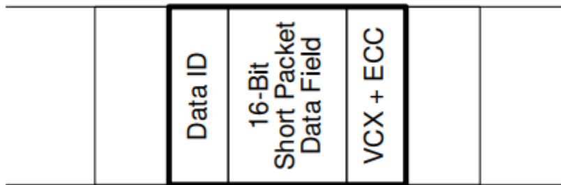
Figure 3-2. MIPI CSI-2 Short Packets
