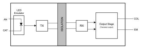
Figure 1-1. ISOM811(0-3)-Q1 Functional Block Diagram
