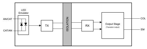
Figure 1-2. ISOM811(5-8)-Q1 Functional Block Diagram
