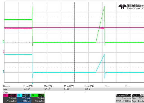
Figure 15. Overcurrent Protection, 0.9-V Output at 12 V_{IN} , 35-A Output (OC_Fault threshold is modified to 35A)
