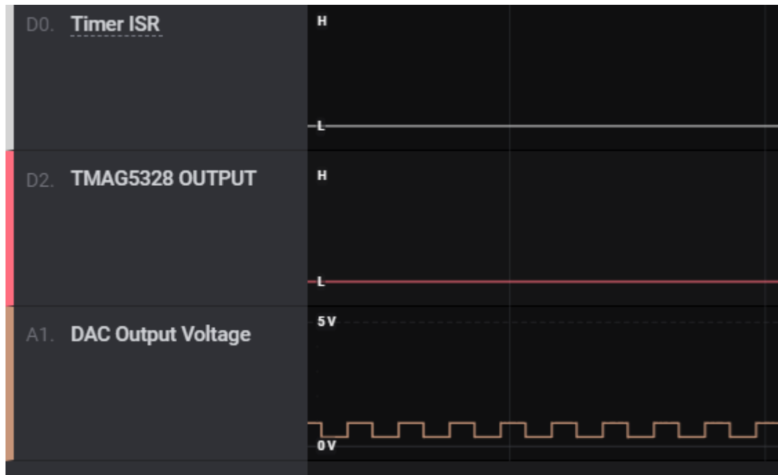
Figure 4-8. Logic Analyzer Screenshot of TMAG5328 OUT Pin When VCC Disconnected
