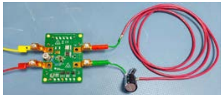
Figure 9. Test setup using the TPS1211-Q1 evaluation module with a 1.5m cable harness.
