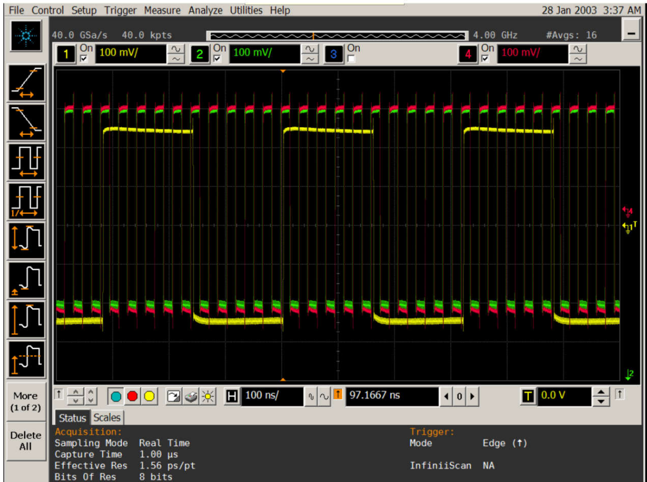
Figure 3-6. Synced Waveforms for Primary, Secondary1, and Secondary2 With Continuous Secondary1 and Secondary2 in Continuous Mode
