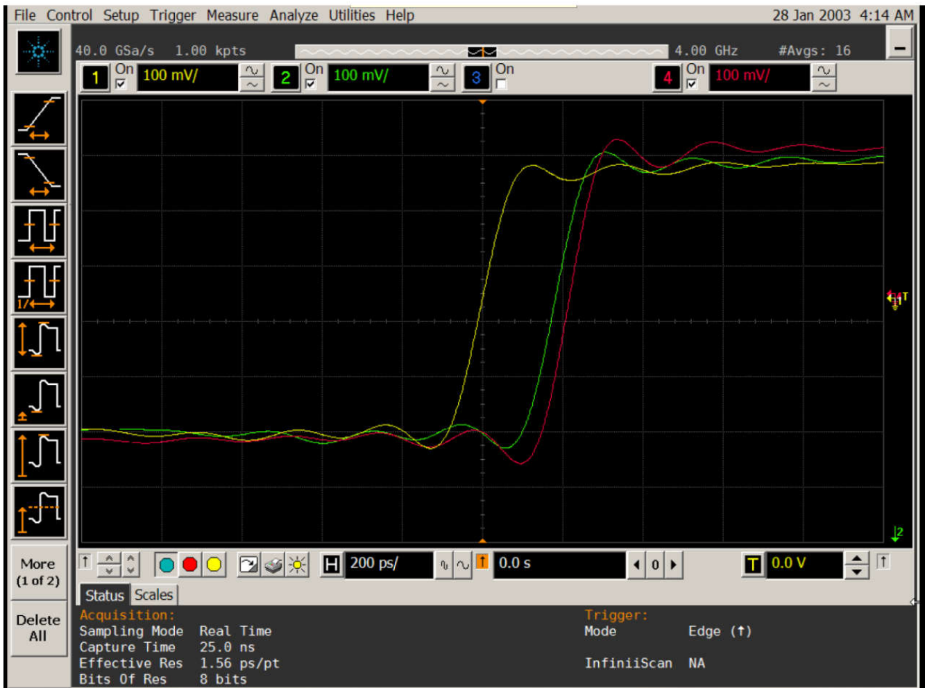
Figure 5-2. Waveforms for Secondary1, and Secondary2 in Repeater Non-sync Mode with Primary in Continuous Mode (Zoomed in)
