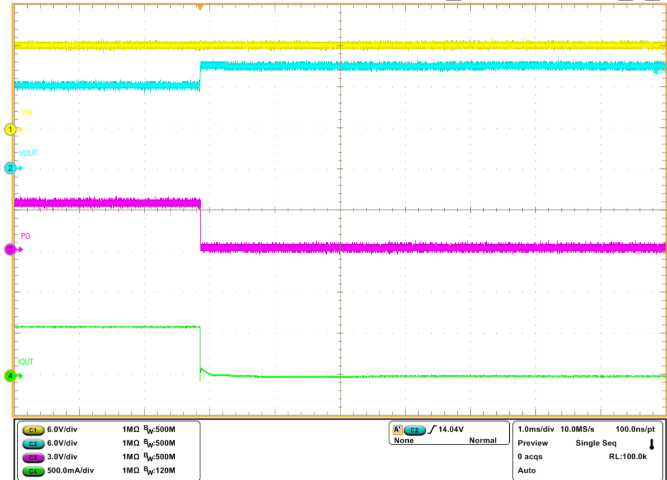
Figure 5-4. Reverse Current Blocking Response of LM73100 Device ( V_{IN} = 12\text{ V} , V_{OUT} = 20\text{ V} )
