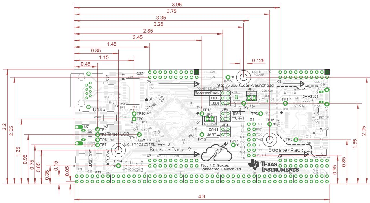
Figure 4-1. Connected LaunchPad Dimensions and Component Locations
