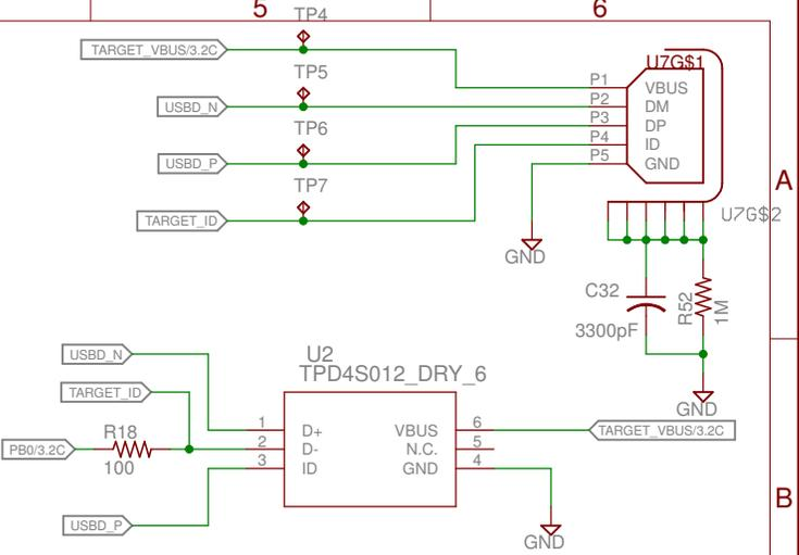
NOTE: TPD4S012 all protection circuits are identical. Connections chosen for simple routing.
