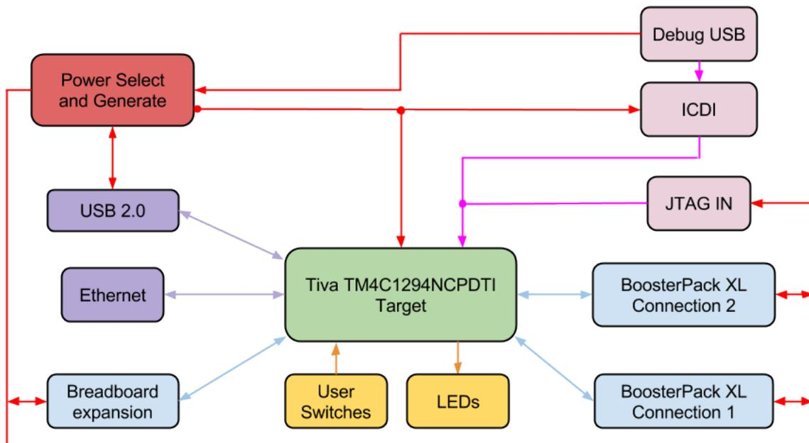
**Figure 2-1. Tiva Connected LaunchPad Evaluation Board Block Diagram**
