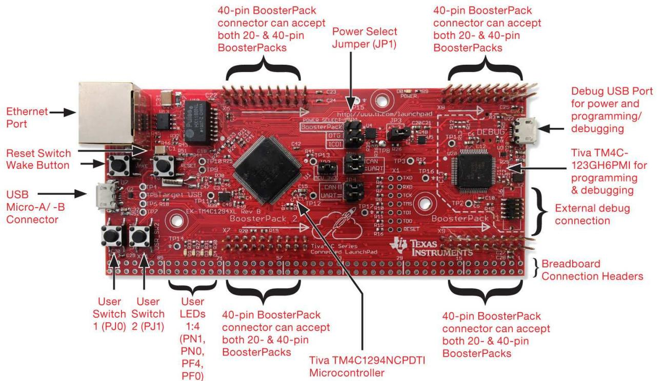
**Figure 1-1. Tiva C Series Connected LaunchPad Evaluation Board**
