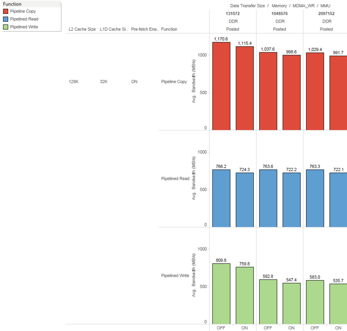
Figure 27. Impact of MMU Enable on DSP RD-WR Performance
