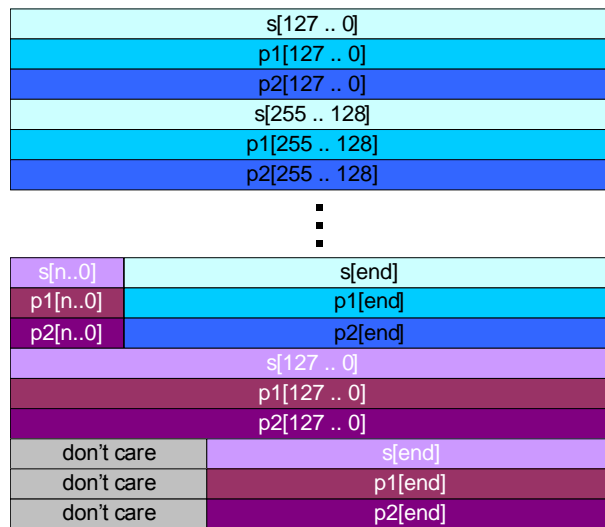
Figure 4-28. Output Format of the Rate 1/3 Convolutional Code and Turbo Code for WCDMA
