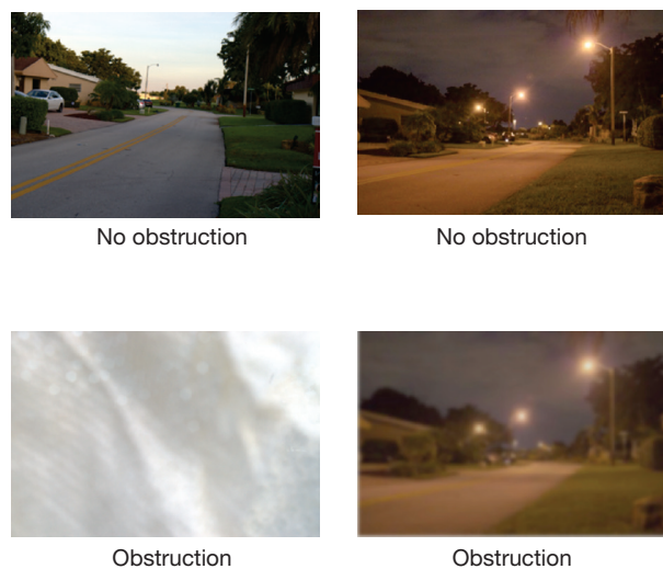
Figure 14. Example of lens obstruction detection.
