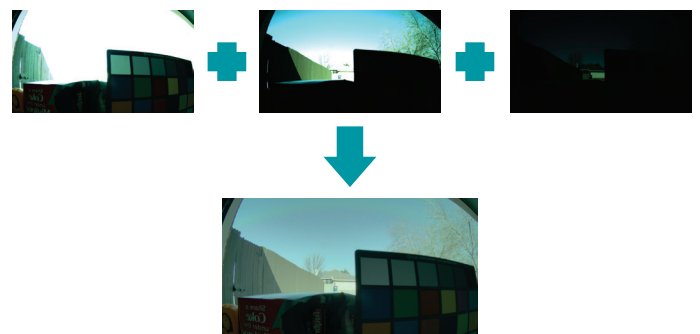
Figure 12. HDR scene construction.
