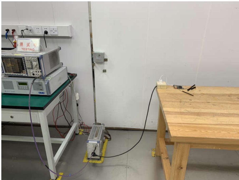
Conducted Emissions Test Setup
