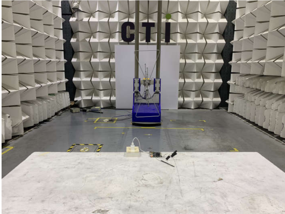
Radiated spurious emission Test Setup-1(Below 1GHz)
