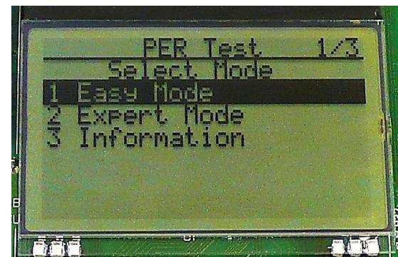
The PER test can be run in several modes. Easy Mode sets up a one-way test and uses default settings. This test is convenient for practical range testing.
