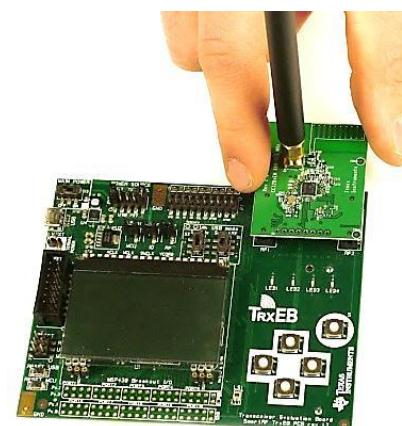
Insert a CC120xEM board into the TrxEB as shown above. Connect the antenna to the SMA connector on the EM.
