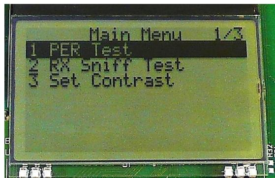
Select the PER (Packet Error Rate) test by highlighting the selection using the up/down buttons. Confirm your selection by pressing Enter (right button).
