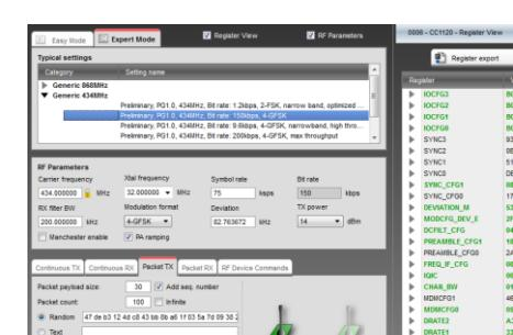
You can now configure the radio, run performance tests, export register settings and run link tests with another CC1200 or CC1201 on a SmartRF TrxEB connected to the PC.
