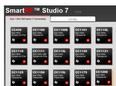
After installing the tool, connect the EB to the PC using the USB cable and start SmartRF Studio. Select the "Sub 1 GHz" tab and double click the highlighted CC1200 device icon.
