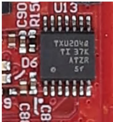
**Figure 2-19. U3 TXU0204-Q1 Level Shifter**
