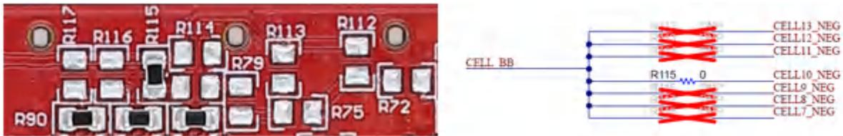
**Figure 2-23. Bus Bar Selection Resistors**
