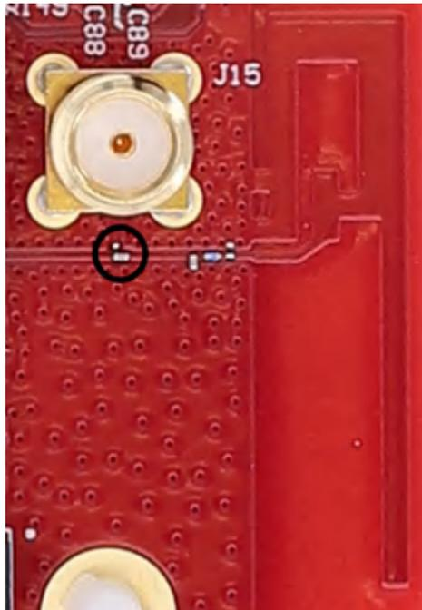
**Figure 2-24. Capacitors for Radiated or Conducted Testing**
