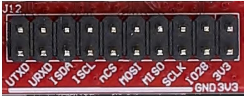
**Figure 2-6. J12 Header for Wireless MCU Interfacing**
