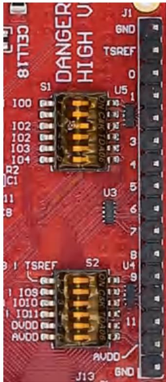
Figure 2-7. BQ GPIO Header
