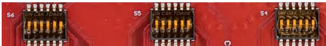
**Figure 2-16. Resistor Ladder Switches**
